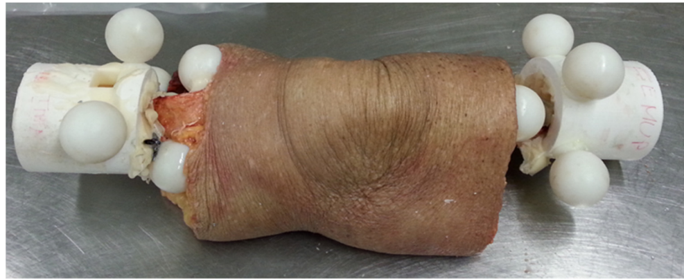
Figure 1. Knee specimen after potting and attaching the fiducial markers. Four or five markers were attached to the potting cup using a nylon threaded stud and two-part resin epoxy glue. Two markers were attached directly to the bone using nylon threaded studs and methylmethacrylate.
