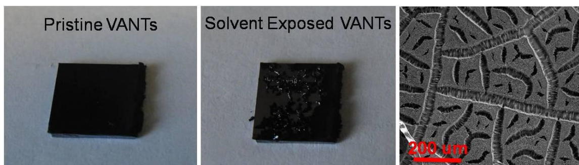
Figure 2-3. VANTs before (left) and after (middle) exposure to ethanol. Solvent exposure results in strong van der Waals forces disturbing the surface to the extent of even pulling the nanotubes away from the substrate. SEM image (right) of a VANT substrate after solvent exposure; a drastic reorganization of the surface is evident.
