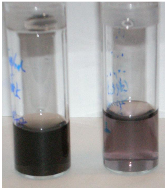
Figure 6-7. Separation of semiconducting SWCNTs by density gradient ultracentrifugation. The less dense purple band (right). The more dense black band containing mostly SWNT bundles(left).
