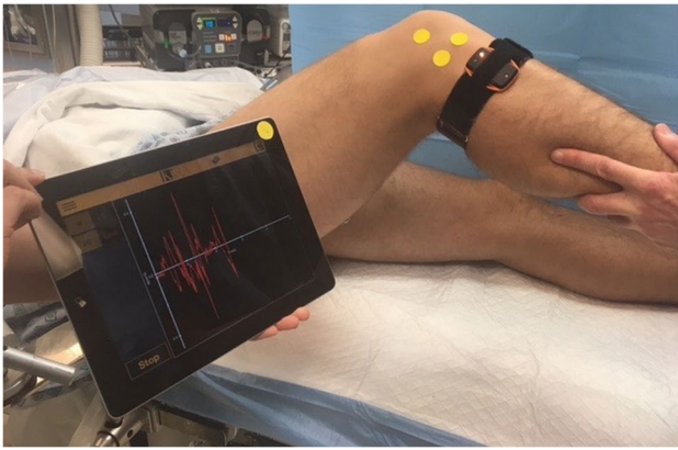
Fig. 2 The KiRa inertial sensor system for quantifying lateral tibial acceleration during the pivot shift test
