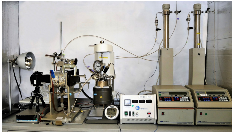
4 Figure 4 High-pressure and temperature contact angle measurement 5 system, (a) Schematic diagram of the system; (b) Photo of the 6 system.
