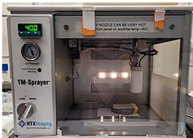
Figure 6. Matrix application configuration TM Sprayer set up for high resolution matrix coating.
