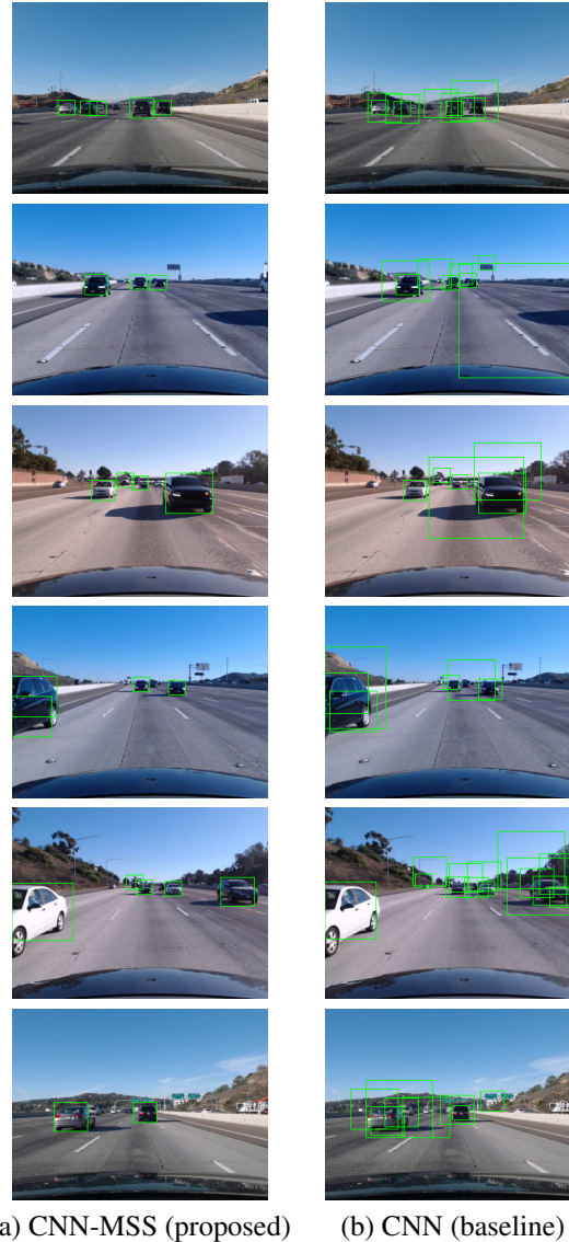
Figure 3.13: Results for vehicle detection on highway settings at a fixed recall rate. Observe how the MSS approach better reasons over multi-scale responses, allowing for higher precision at the same recall rate and better localization compared to the single-scale CNN, which employs independent scoring at each scale and relies on NMS alone for resolving multi-scale responses.
