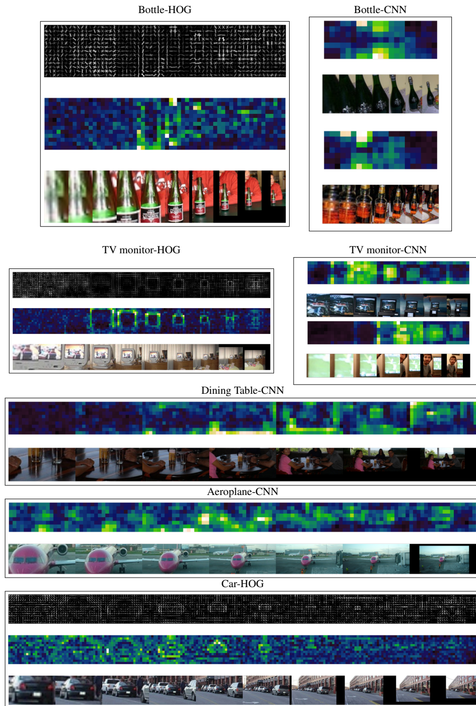
Figure 3.5: Visualization of multi-scale CNN and HOG templates. For each model, the maximum positive SVM weight for each block is shown together with an example instance. Brighter colors imply higher discriminative value. Large amount of discriminative value is placed at nearby and remote scales corresponding to contextual information (e.g. road cues at other scales).
