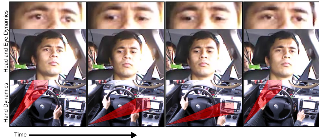
Figure 5.1: Hand, head, and eye cues can be used in order to analyze driver activity. Notice the guiding head movements performed in order to gather visual information before and while the hand interaction occurs.
