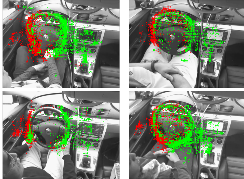
Figure 4.23: Visualizing hand locations of entire drives. In red are left hand positions and in green are right hand positions. The scatter plots above show several hours of collected video.
