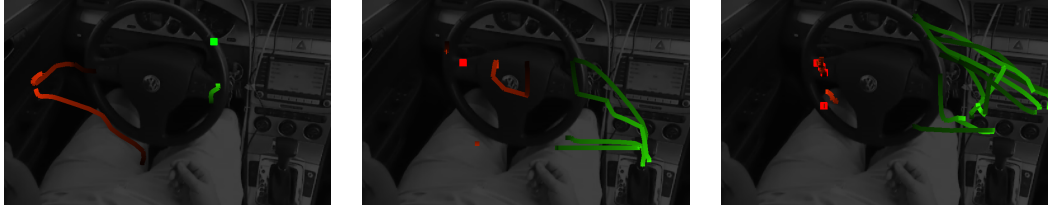
Figure 4.24: A dataset of transition reaching and retracting gestures is used for the experiments. Left hand trajectories are shown in red and right hand trajectories are shown in green. Trajectory color encodes time, with brighter being more recent in the trajectory. Shown are reaching gestures to left side rest, gear, and instrument cluster.
