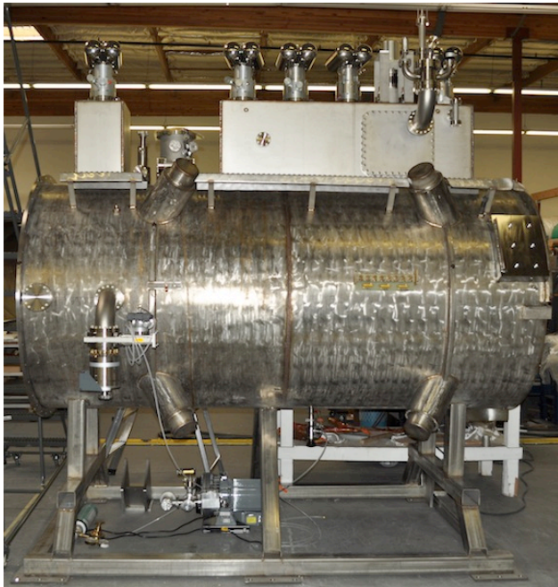
Figure 6: Completed reassembly of first magnet.
