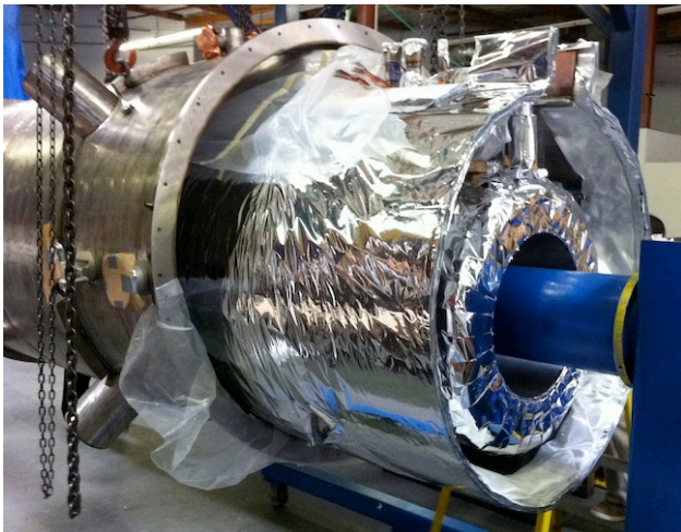
Figure 3: Assembly of shield/cold mass into cryostat.
