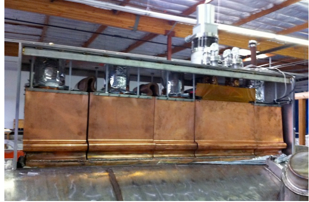
Figure 4: Improved shield connection to cryocoolers.
