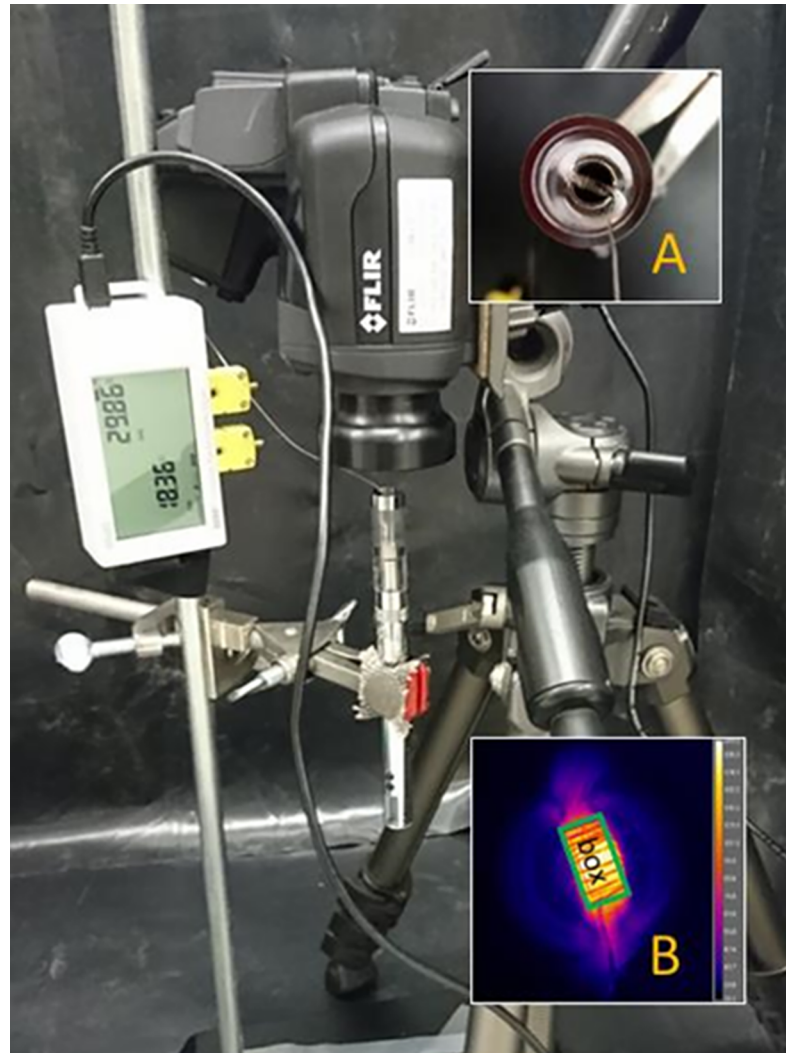
Fig 1. Experimental setup for determination of coil heating temperature using a thermocouple and an infrared (IR) camera: (A) typical position of the thermocouple on a coil head; and (B) details of the heating coil section (green box) from which minimum, mean, and maximum temperatures were determined using an IR camera.
