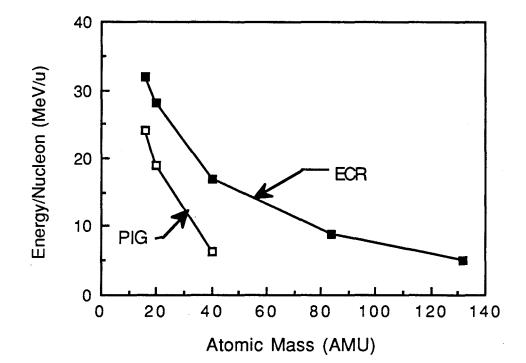
1. Energy vs. mass using PIG and ECR sources, with 10<sup>10</sup> particles/sec cyclotron external beam.
