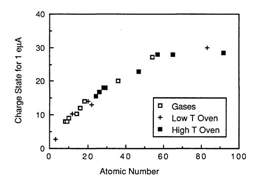
4. Charge states for 1  $e\mu A$  intensity from the ECR source for gas and solid material feed.
