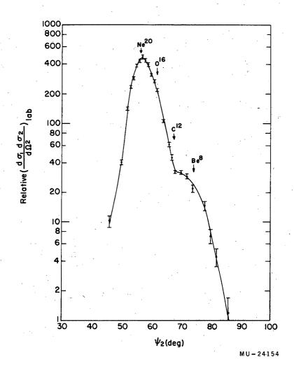
Fig. 10. Fission-fragment angular correlation for the system 207-Mev Ne $^{20}$ +Bi $^{209}$ .  $\psi_1$  at 90 deg. Each arrow represents the estimated peak position for the capture of the indicated fragment from the incident heavy ion.
