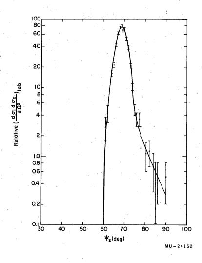
Fig. 8. Fission-fragment angular correlation for the system 110-Mev  $0^{16}$ + $U^{238}$ .  $\psi_1$  at 90 deg.
