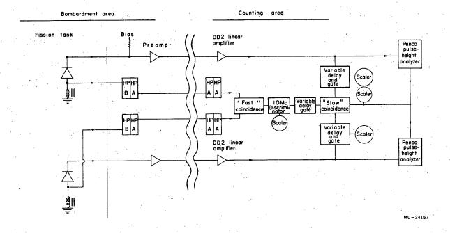
Fig. 2. Electronic system used in the angular correlation experiments.
