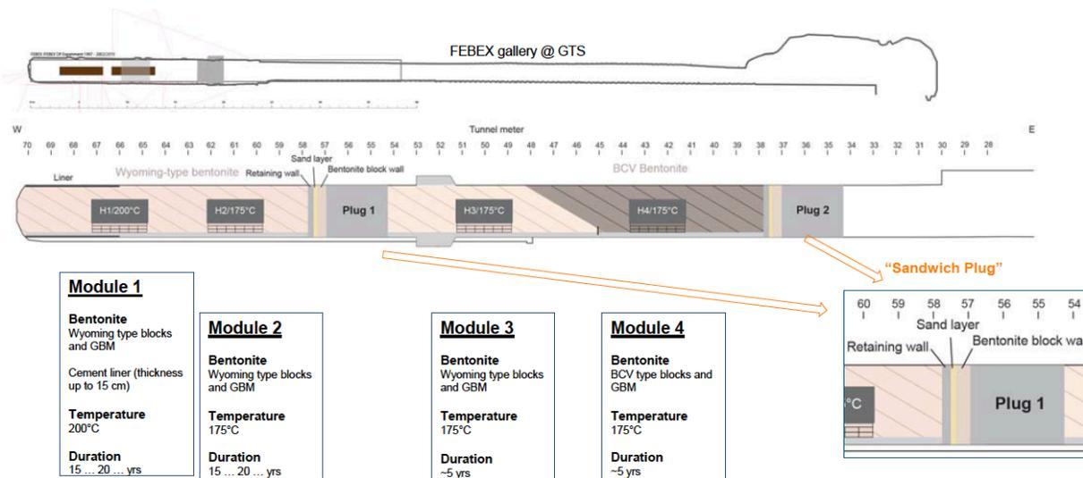
Figure 3.3-5. Final HotBENT design with individual modules (Kober, 2020).
