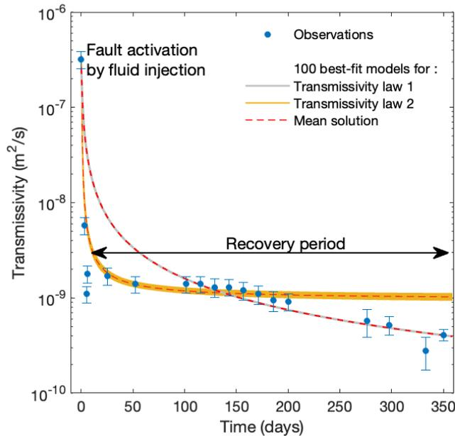
**Figure 3.1-15. Evolution of predicted fault transmissivity over time compared to experimental data estimated from the series of pulse tests. Experimental results are shown as blue dots with error bars taken at  $\pm 20\%$  to account for possible uncertainty of measurements. Two fault transmissivity laws are deployed, shown in gray and orange. Source: Rutqvist et al. (2024a, Section 8.2.3.2).**
