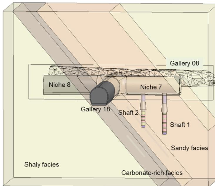
Figure 3.2-19. Schematic of the two shaft geometries in the SANDWICH experiment (Friedenberg et al., 2023).
