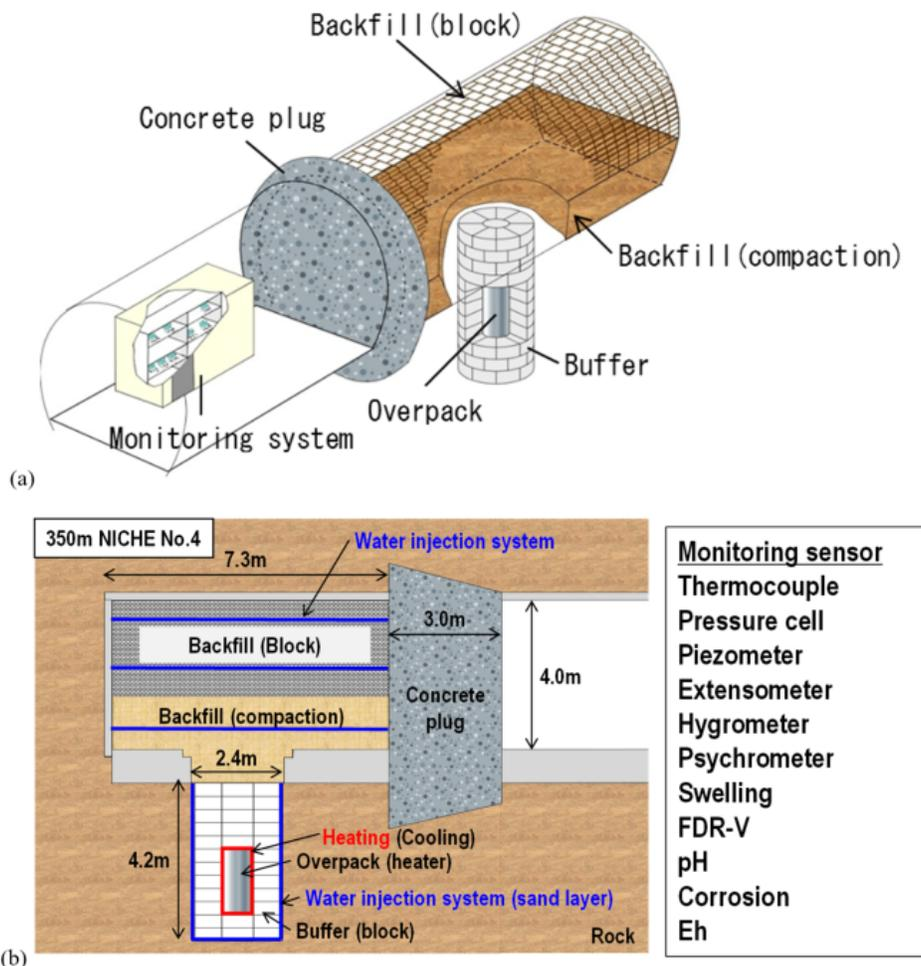
Figure 3.2-6. Schematic view of the Horonobe full-scale *in-situ* EBS experiment (Bond and Birkholzer, 2019). (a) 3D setup and (b) cross-section.
