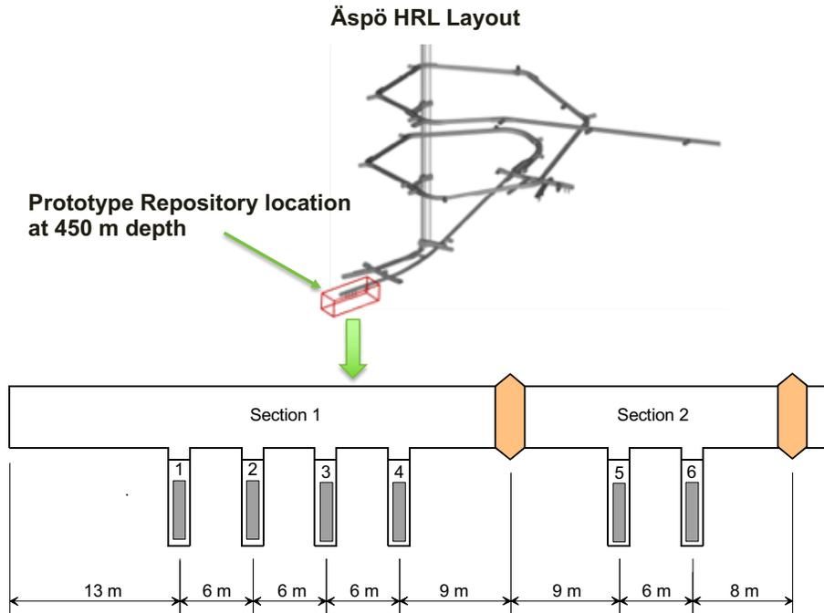
Figure 3.4-5. Äspö HRL layout and configuration of the Prototype Repository test (modified from Svemar et al., 2016).
