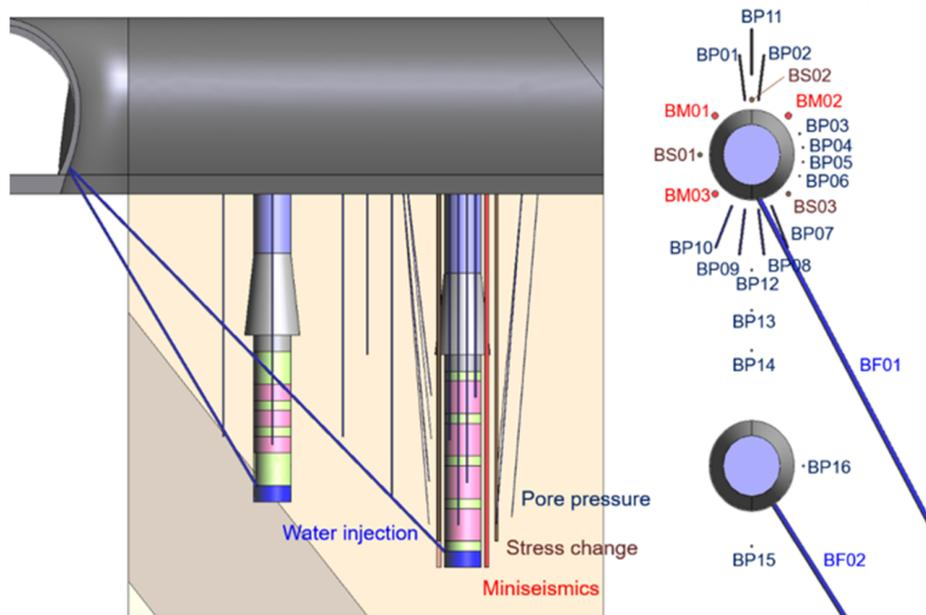
Figure 3.1-18. Design of SW-A experiment with two vertical shafts and planned monitoring approach (Hesser and Wiezcorek, 2020).
