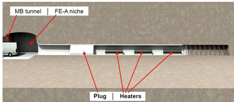
Figure 3.1-6. FE Heater Test: Side view of the experiment setup and the heater layout (Garitte, 2010).
