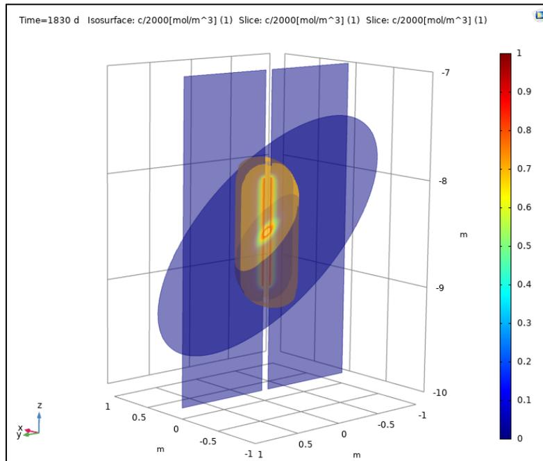
Figure 3.1-23. Scoping simulations of tracer diffusion in heated Opalinus Clay as per DR-C design (Bernier and De Canniere, 2020).
