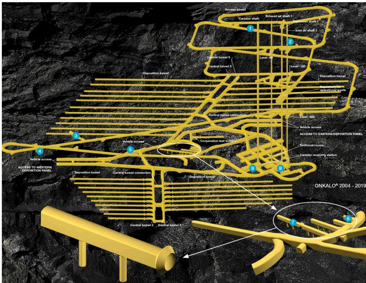
Figure 4.9-1. Layout of the Onkalo URL in Finland. Numbered areas 1-5 are research niches, 6-9 are demonstration tests and other tests. Source: Jalonen (2024).
