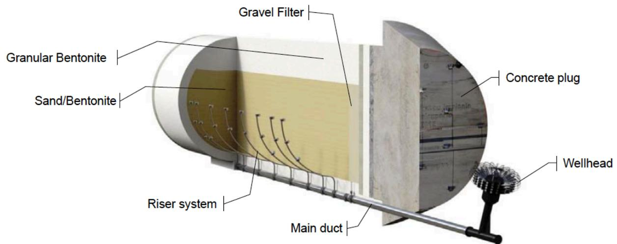
Figure 3.3-10. Schematic illustration of Gas Permeable Seal Experiment at GTS (Reinicke et al., 2020).
