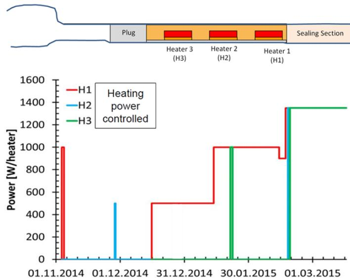
Figure 3.1-9. Heat power applied to Heaters H1, H2, and H3 during the start-up of heating at the Mont Terri FE experiment.
