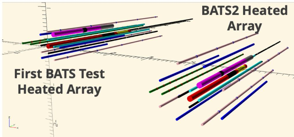
Figure 3.2-18. Schematic of borehole setup for first BATS test versus BATS2 (Kuhlman, 2023).
