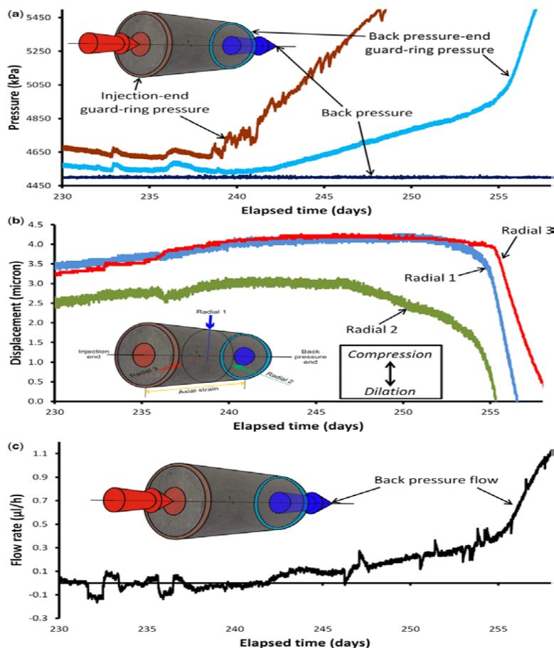
Figure 3.1-19. Data from a triaxial test report by Cuss et al. (2014) showing the response of a claystone sample at the onset of gas flow: (a) pressure response; (b) radial deformation; (c) outflow from the sample.
