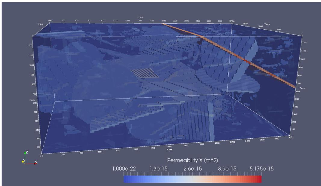
**Figure 3.2-11. Generic reference case for a crystalline repository as developed by the SFWST campaign. The figure shows emplacement 3,360 waste packages in 168 drifts placed 20 m apart, with a fracture network based on Forsmark (Sweden) fracturing characteristics (Stein, 2020).**
