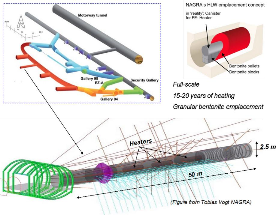
Figure 3.1-5. FE Heater Test at Mont Terri URL: experiment setup and borehole layout (Zheng et al., 2015).
