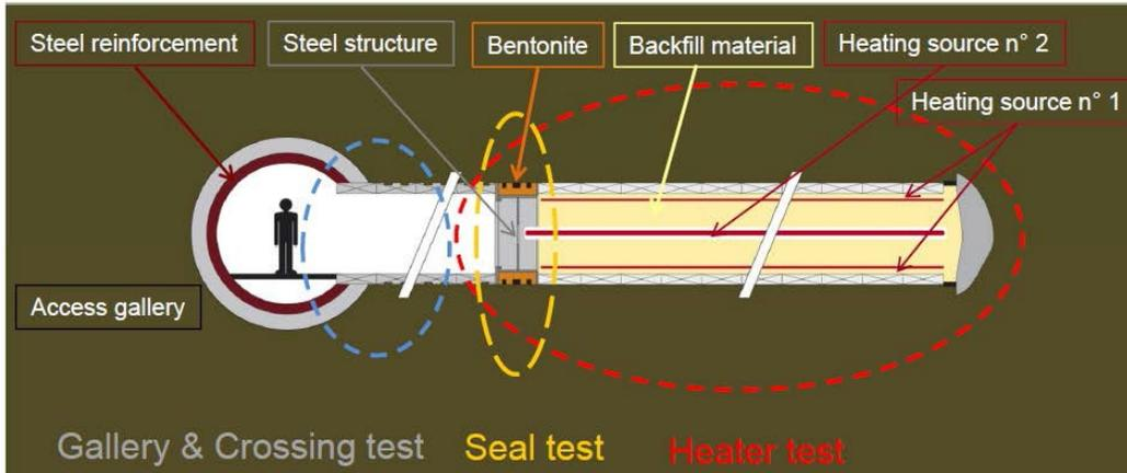
Figure 4.8-2. Layout of the PRACLAY *in-situ* experiment at HADES URL (Li, 2011).
