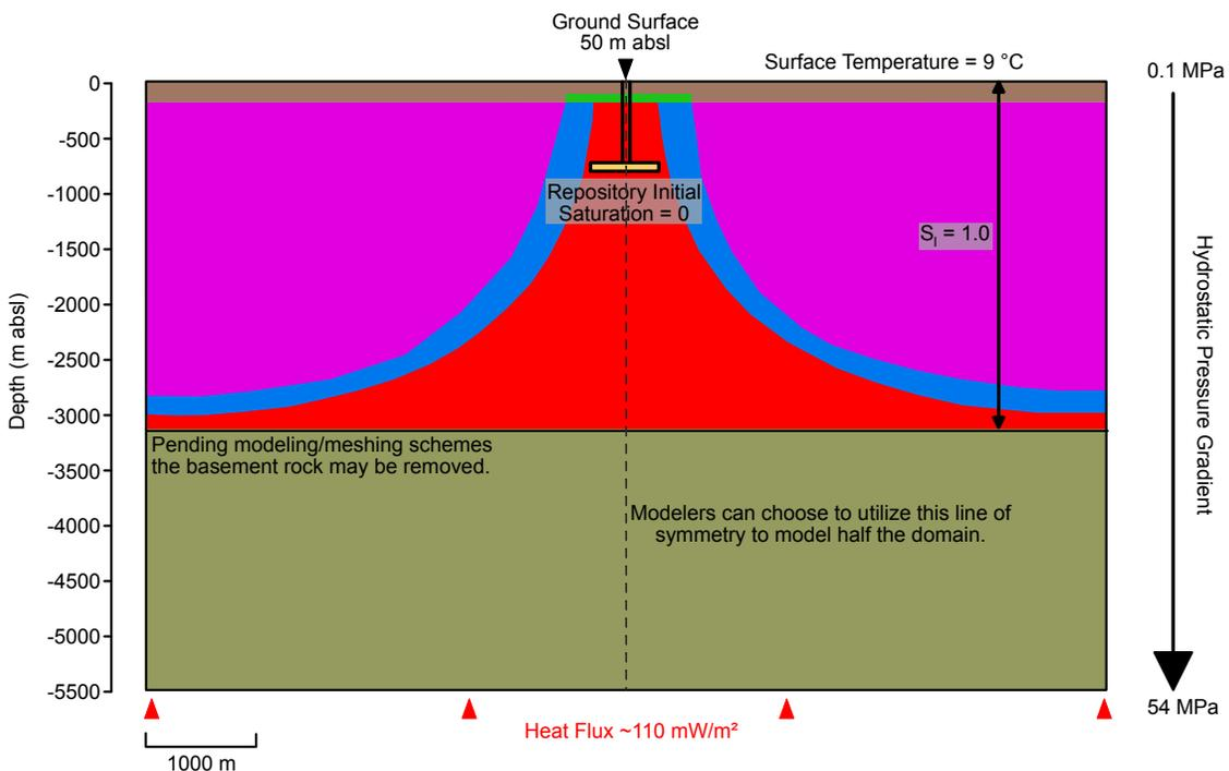
Figure 3.2-23. Generic reference case for a salt repository as developed by the SFWST campaign (Mariner and Jayne, 2023).
