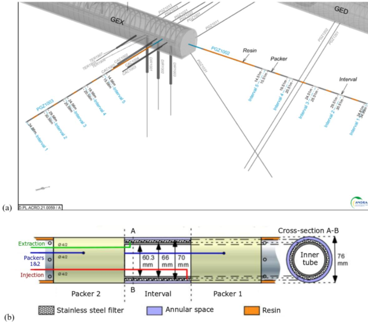
Figure 3.2-3. (a) Borehole setup for gas fracturing *in-situ* experiment (PGZ). (b) Multi-packer system for injection tests. Source: Plúa and Armand, 2020.
