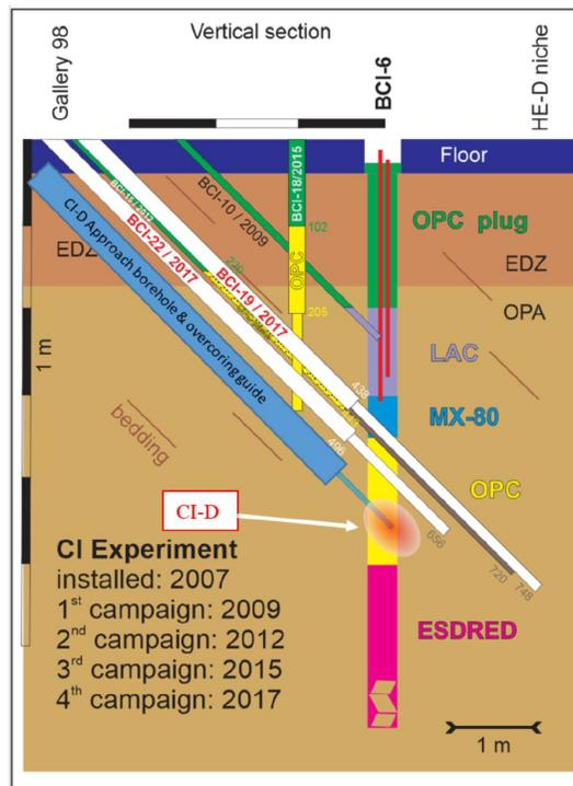
Figure 3.1-17. Schematic of CI-D experiment (Maeder and Martin, 2022). The CI-D overcoring borehole is approaching the zone of long-term interaction between OPC and the OPA. Note that the bedding within the OPA is parallel to the overcoring borehole and at an angle of about 45° from the contact with the cement plug. First, information from the overcoring is expected to be available in 2024.
