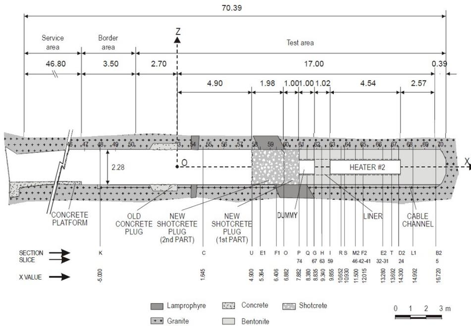
Figure 3.3-3. *In-situ* test configuration following dismantling of Heater 1 (Huertas et al., 2005).
