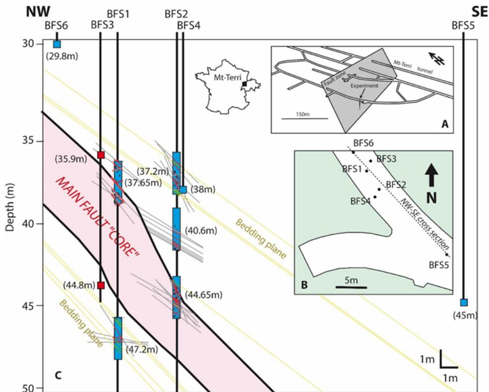
Figure 3.1-12. Test intervals across the Mont Terri Main Fault (red squares are seismic sensors, blue squares are piezometers, blue rectangles are injection and monitoring intervals); (a) experiment location in Mont Terri URL; (b) map of the borehole geometry in the FS experiment zone; and (c) cross-section showing the different testing intervals.
