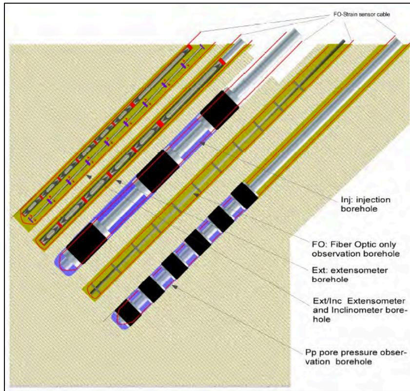
Figure 3.1-20. Schematic showing the field test design with central gas injection borehole surrounded by monitoring boreholes.
