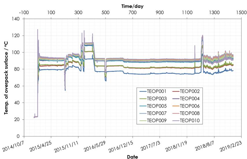
Figure 3.2-7. Temperature evolution in the EBS experiment (Sugita, 2020).
