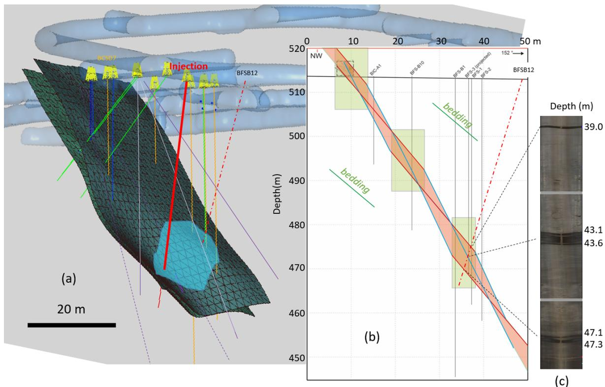
Figure 3.1-13. 3D setup of the FS-B/FS-C experiment. (a) Main fault top and bottom surfaces. (b) Geological cross-section showing the schematic internal structure of Asperities. (c) Post 2021 injection experiment coring through the Main Fault showing three wet zones corresponding to preferential flow paths created during the experiment.
