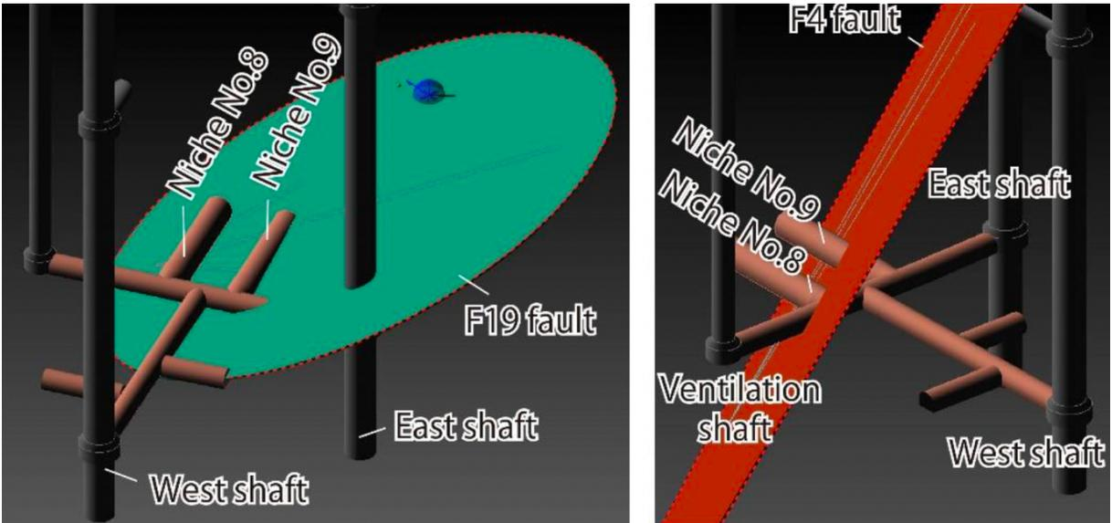
Figure 3.5-3. Predicted fractures in and around the 500 m Niches No. 8 and No. 9.
