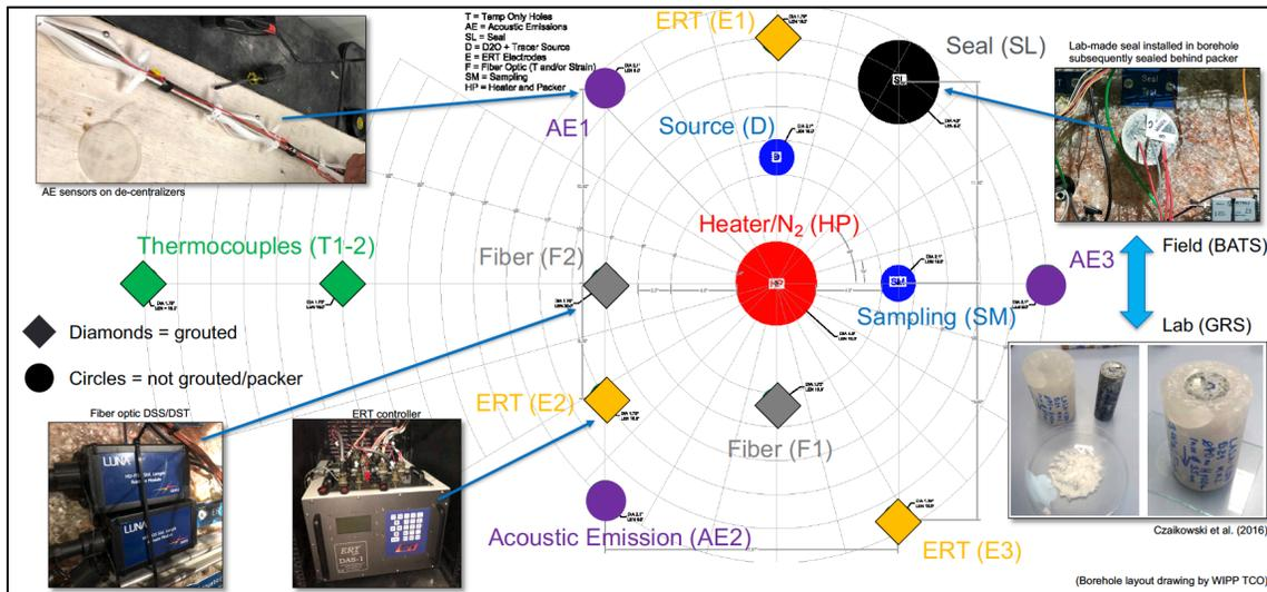
Figure 3.2-10. Borehole layout with a central heater borehole and satellite monitoring boreholes in a vertical cross-section perpendicular to the heater element (Kuhlman, 2020).
