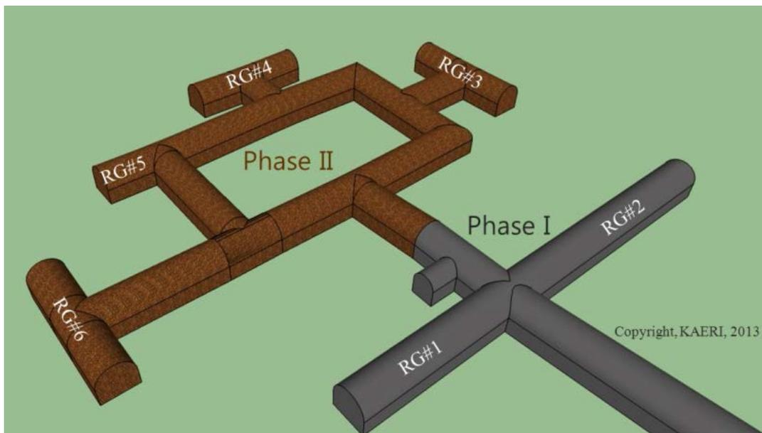
Figure 4.2-2. Layout for tunnel extension of KURT (Wang et al., 2014).
