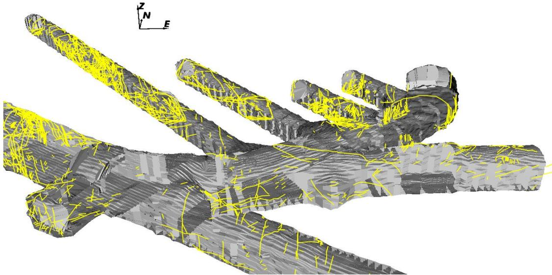
Figure 3.2-21. Fracture traces mapped in the Demonstration Area at Olkiluoto (Geier et al., 2023).
