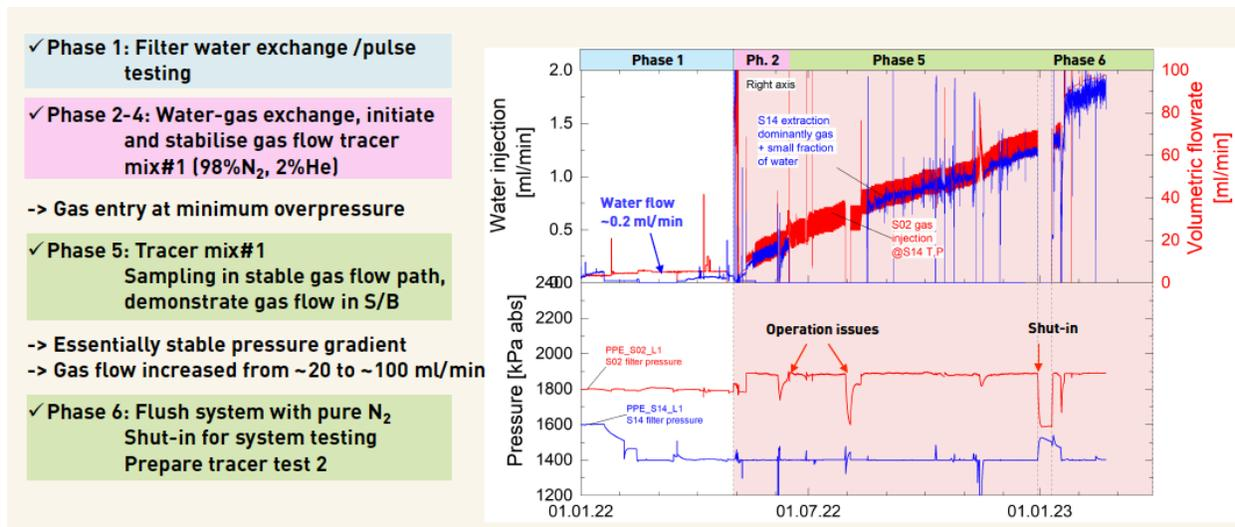
Figure 3.3-11. Phases 1 to 6 in the GAST, and measured water injection rate, gas flow rate, and pressure (Spillmann et al., 2023).
