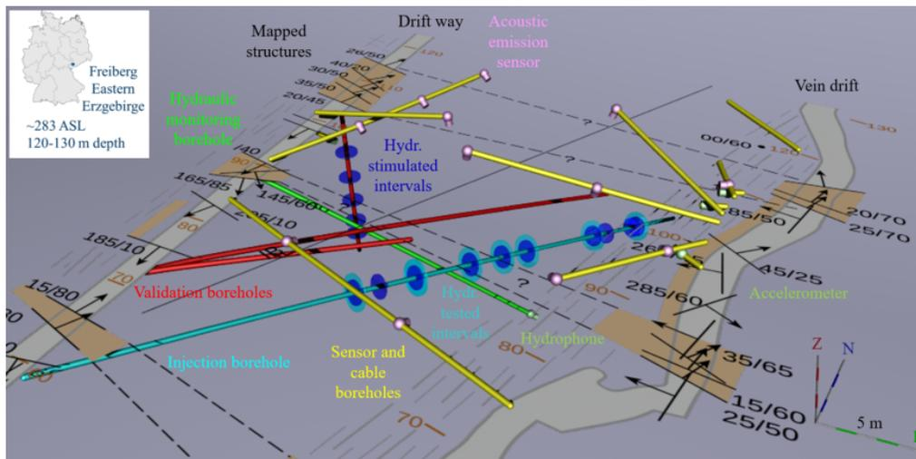
Figure 3.2-15. Schematic of STIMTEC stimulation experiment (Kolditz, 2023).
