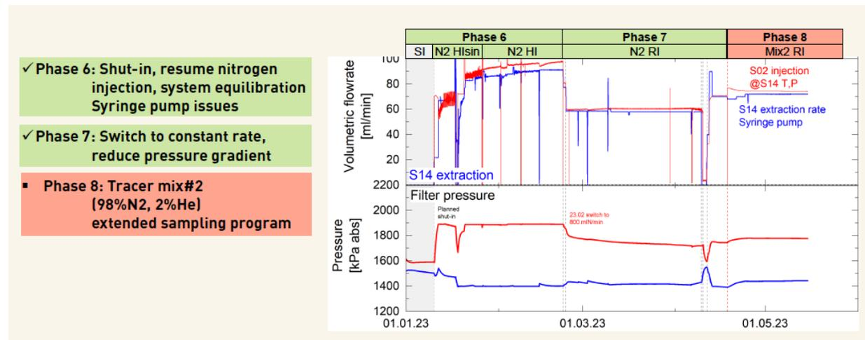
Figure 3.3-12. Phases 6 to 8 in the GAST, and measured water injection rate, gas flow rate, and pressure (Spillmann et al., 2023).
