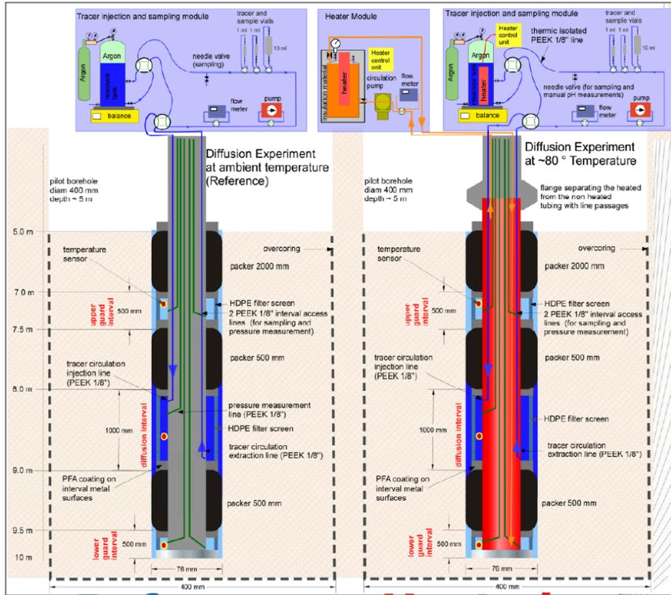
Figure 3.1-22. Schematic showing DR-C design with heated (right) and unheated (left) setups (Bernier and De Canniere, 2020).
