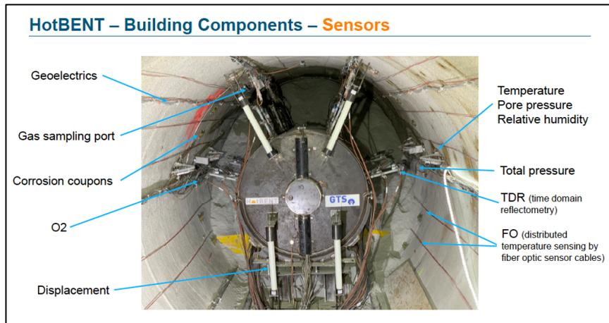
Figure 3.3-6. Photo showing the heater and sensor equipment in the HotBENT tunnel (Kober, 2021).
