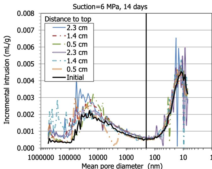
Figure 3.4-4. Incremental intrusion of pelleted bentonite swelling into a gap (Gens, 2021).
