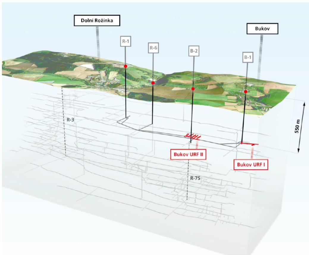
Figure 4.10-1. Schematic layout of the research areas in the Bukov URF (from Dohnálková, 2024).
