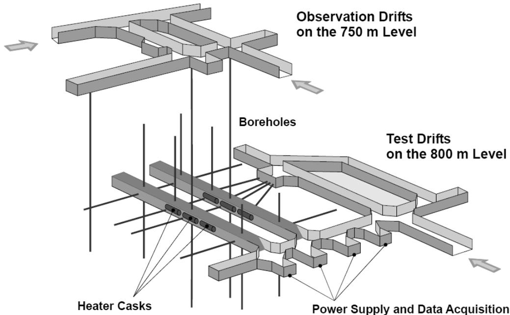
Figure 4.1-2. Schematic view of the two drift tests used in the TSDE experiment (800 m level of the Asse salt mine) (Rutqvist et al., 2015).
