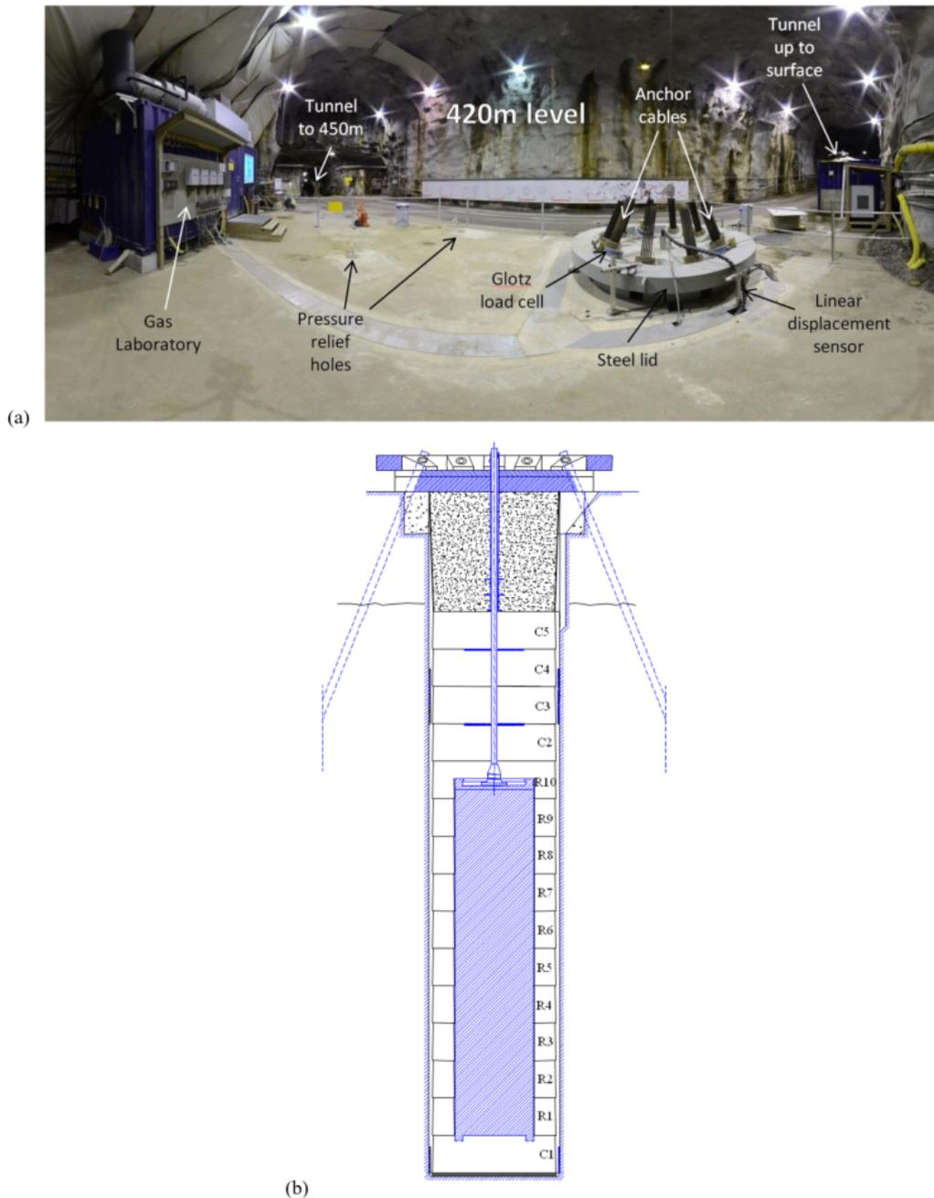
Figure 3.2-4. Large-Scale Injection Test LASGIT at Äspö HRL (Harrington and Tamayo-Mas, 2020). (a) Photo of the LASGIT installation at the 420 m level; and (b) cross-section of LASGIT setup in vertical deposition hole. There are ten filter levels R1 – R10 that have been used for segmented gas injection tests.
