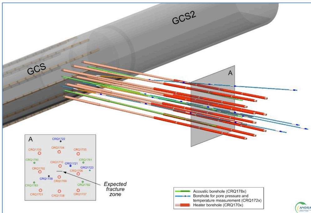
Figure 3.2-2. Borehole setup for CRQ thermal fracturing experiment (Plúa and Armand, 2020).
