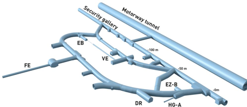
**Figure 3.1-1. 3D schematic of the Mont Terri URL with side galleries and drifts. This schematic does not show the recently finalized expansion of the URL. Abbreviations point to some of the key experiments conducted at Mont Terri.**
