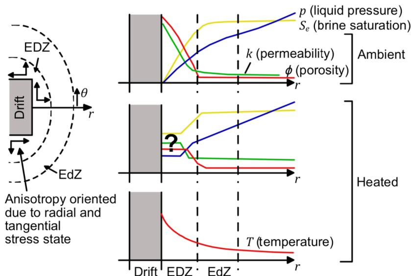
Figure 3.2-8. Schematic trends in hydrological properties and state variables from a drift in salt to the far field under ambient (top) and heated (bottom) conditions (Kuhlman, 2020).
