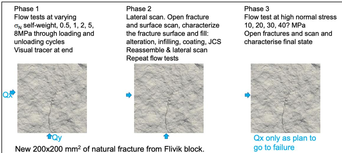
Figure 3.4-3. HM testing conducted for Task 10.2 (Bruines and Lanyon, 2021).
