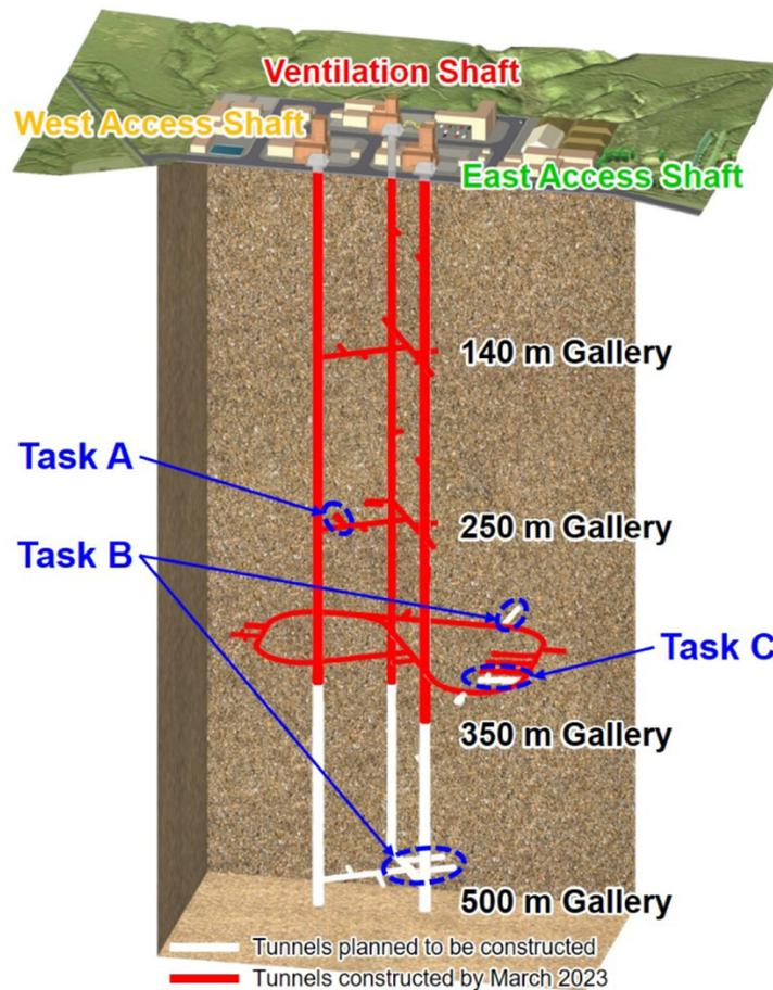
Figure 3.5-1. 3D schematic of the Horonobe URL in Japan.
