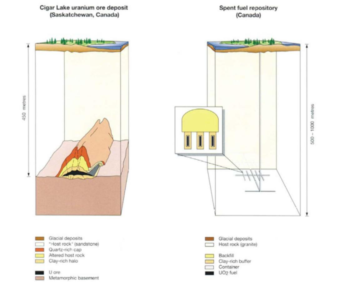
Figure 3.2-22. Schematic of the Cigar Lake Analog versus deep geologic disposal (Nguyen and Li, 2023a).
