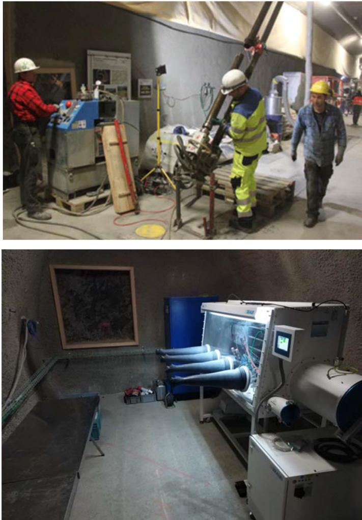
Figure 3.1-21. Borehole BMA-A1 (top) and glovebox in side alcove (bottom) of MA-A experiment.
