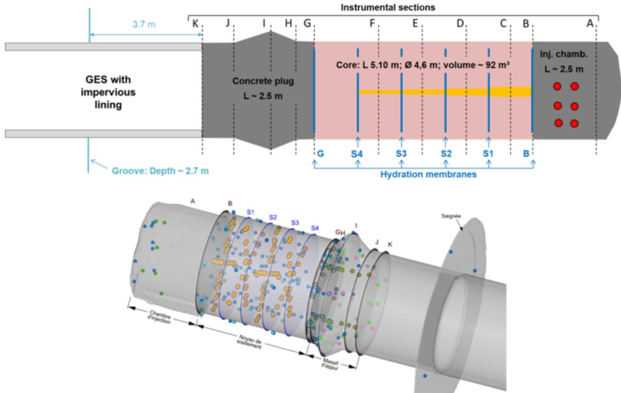
Figure 3.2-20. Top: Schematic showing the seal testing section of the NSC experiment situated between two concrete plugs. Bottom: Sensor locations for pressure and saturation (Plúa and Armand, 2023).
