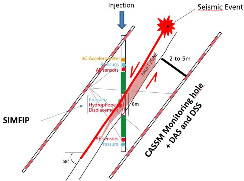
**Figure 3.1-14. Vertical cross-section showing a schematic of tilted boreholes for cross-well geophysical monitoring of the dynamic fault behavior upon activation.**
