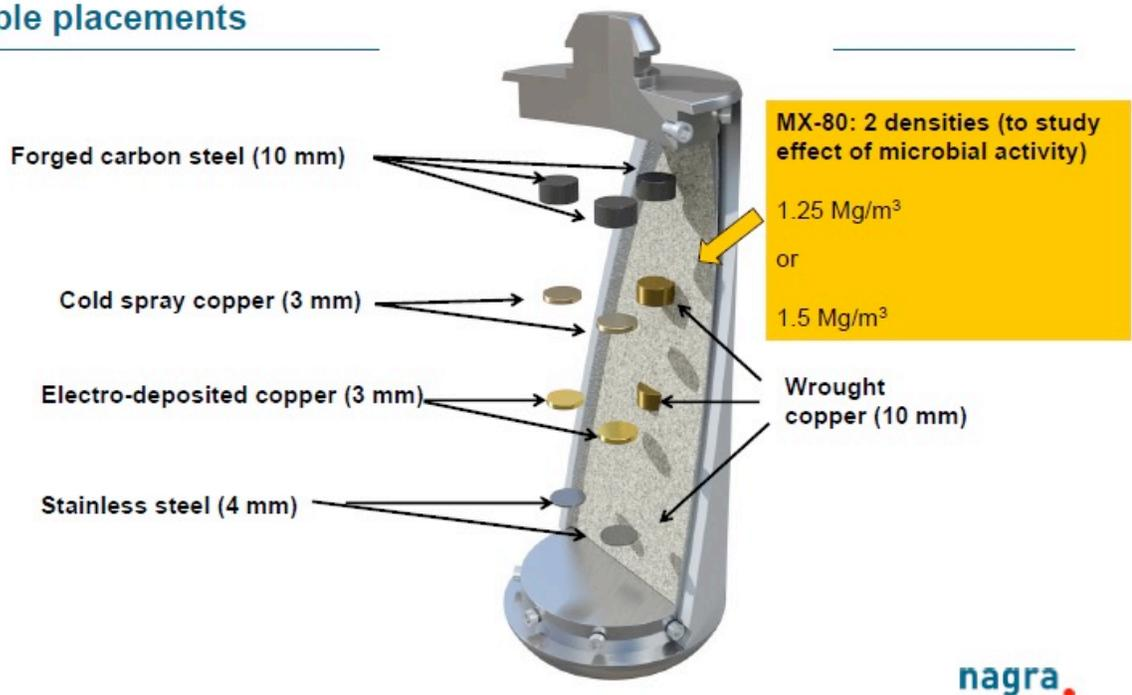
Figure 3.3-14. Schematic illustration of MaCoTe Experiment at GTS (Martin, 2022).
