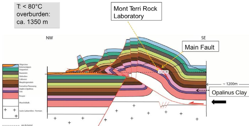
Figure 3.1-10. Geologic setting showing Mont Terri URL and location of the main fault (Guglielmi et al., 2015).
