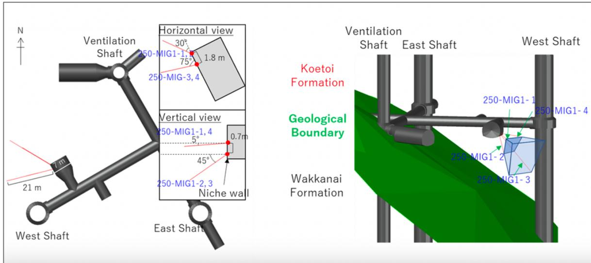
Figure 3.5-2. Layout of the four boreholes for the tracer experiments planned at the 250 m Gallery.
