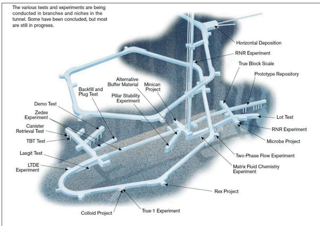
Figure 3.4-1. The layout of Äspö HRL and location of main experiments (Birkholzer, 2012).
