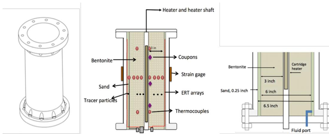
Figure 3.3-8. Schematic diagram of the column design for HotBENT-Lab #2 experiment. Left: 3D rendering of the column exterior; Middle: interior design of the bentonite column showing locations of sensors and the heater; Right: water flow port on the end cap. Tracer particles and coupons are shown at representative locations (Zheng et al., 2022).
