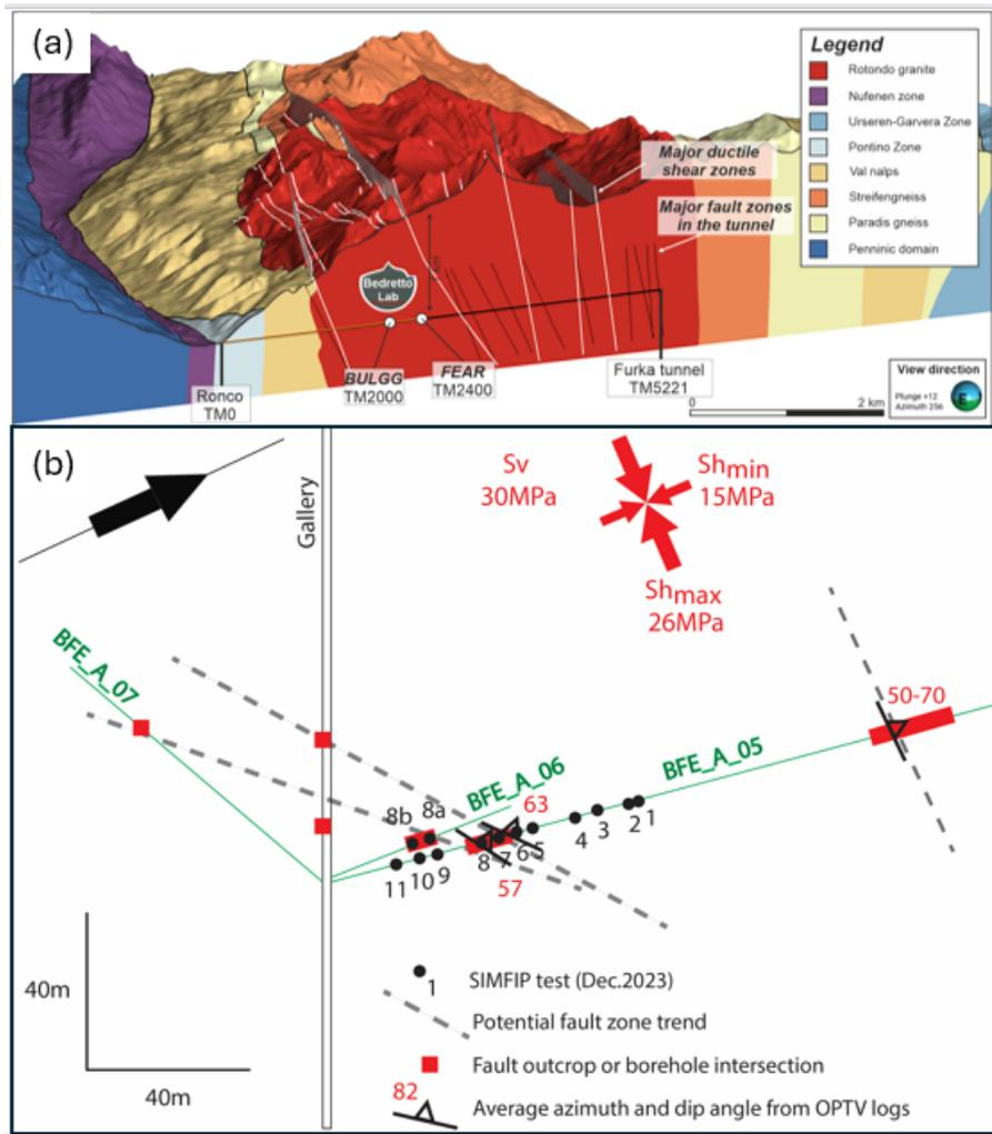
Figure 4.4-1. (a) Bedretto underground laboratory with the FEAR tests set in the Rotondo granite in Switzerland. (b) A detailed map shows the boreholes (green lines) drilled across the fault zone. Black dots with numbers 1 to 11 show the SIMFIP tests conducted in borehole BFS-A-05 to estimate stress variations across the fault zone (grey dashed lines) and fault properties (Hu et al., 2024).
