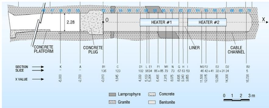
Figure 3.3-2. Schematic cross section of the FEBEX Test at Grimsel Test Site (Nagra, 2014).
