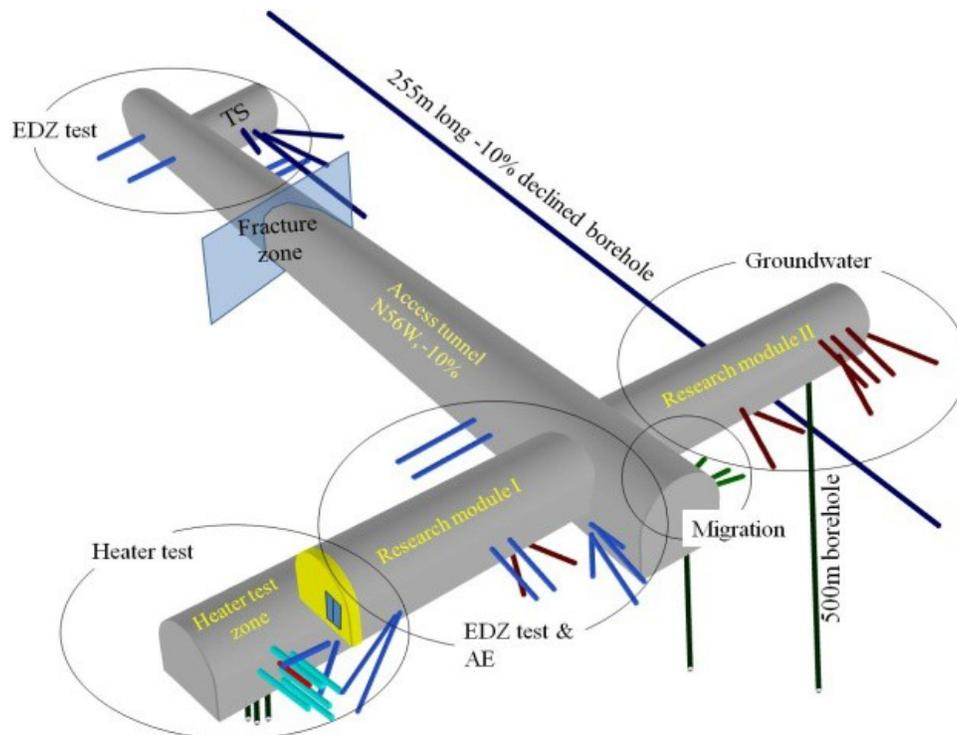
Figure 4.2-3. Location of *in-situ* tests and experiments at KURT (from Wang et al., 2014).
