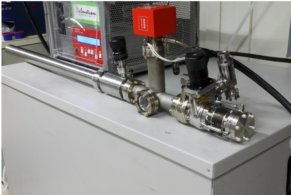
Figure C.1: The ALS vacuum suitcase and its power supply
