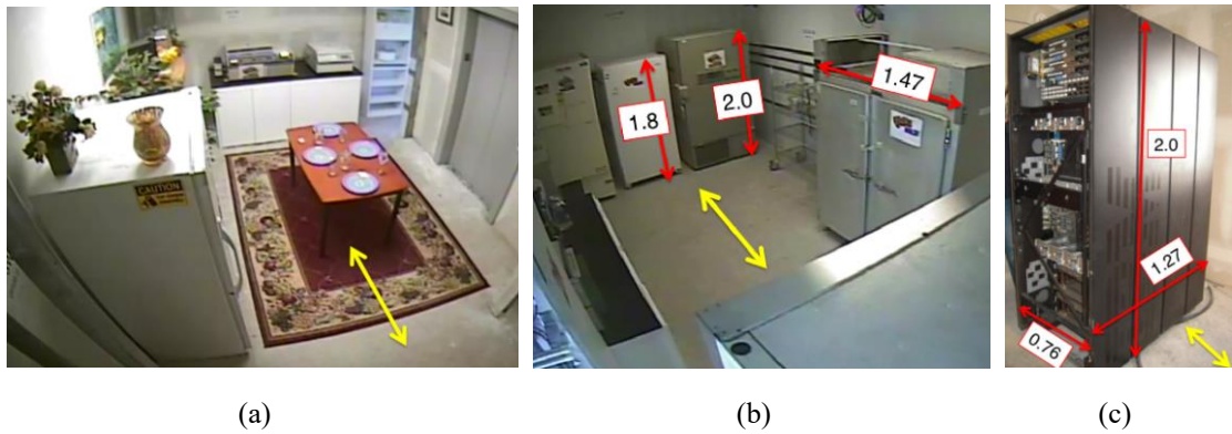
Figure 2.7: (a) Residential and (b) laboratory space on level two. (c) Computer server on level three. Arrows on slab indicate direction of input motion. Units: meters.
