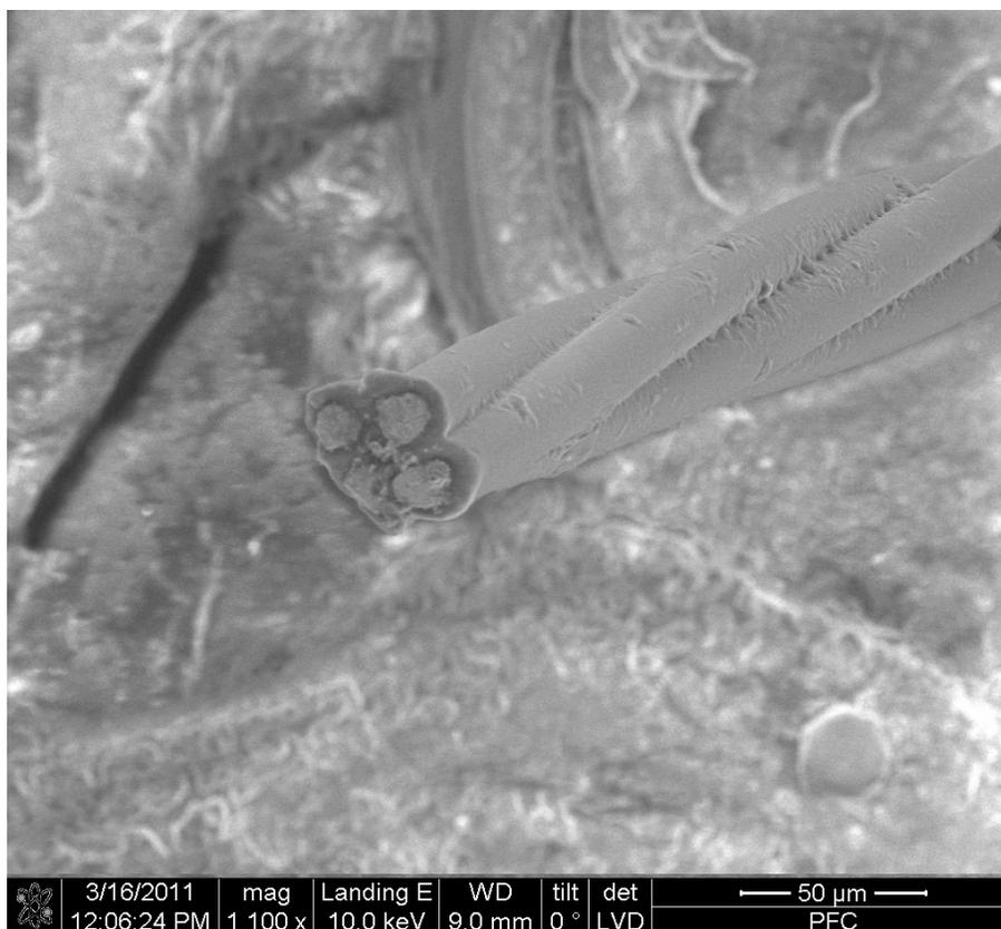
Figure 1.1: Scanning electron microscope image of a tetrode probe. Four  $13 \mu\text{m}$  nichrome electrodes are twisted together and the insulation fused with a heat gun.
