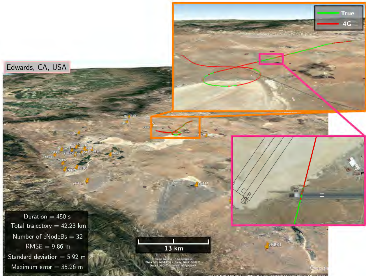
Figure 5.29: High-altitude aircraft navigation – Region A: Edwards, CA, USA – Experimental environment and aircraft navigation results showing: eNodeB positions, true aircraft trajectory, and aircraft trajectory estimated exclusively using cellular 4G signals. The aircraft traversed a total distance of 42.23 km traversed in 450 s during the experiment. The position RMSE over the entire trajectory was 9.86 m.
