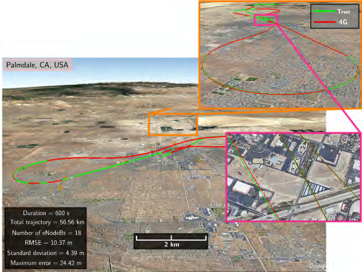
Figure 5.32: High-altitude aircraft navigation – Region B: Palmdale, CA, USA – Experimental environment and aircraft navigation results showing: eNodeB positions, true aircraft trajectory, and aircraft trajectory estimated exclusively using cellular 4G signals. The aircraft traversed a total distance of 56.56 km traversed in 600 s during the experiment. The position RMSE over the entire trajectory was 10.37 m.
