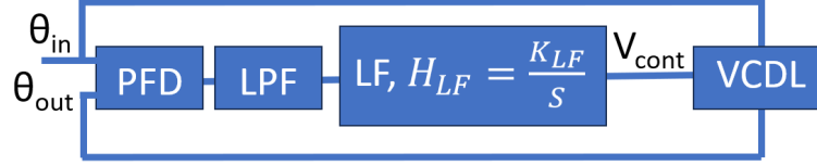
Figure 2.17: A linear model for the DLL. The PFD and LPF blocks model the costas PFD. The LF is modeled as an ideal integrator. The voltage controlled delay line (VCDL) adjusts the output phase based on the input voltage.
