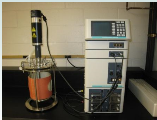
Figure 1: Continuous cultivation of model communities was performed using bioreactors such as the New Brunswick Bioflo 110.
