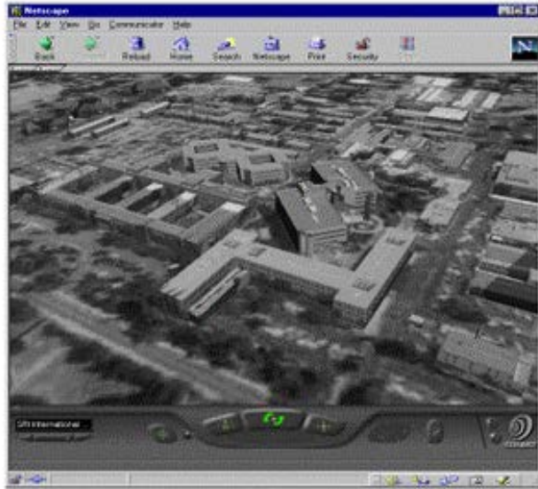
Figure 8. A texture-mapped site model of the SRI International campus that has been georeferenced onto an underlying terrain model. Note the accurate alignment of the latitude/longitude-specified buildings with the underlying 1 m resolution USGS DOQ satellite imagery in UTM coordinates.
