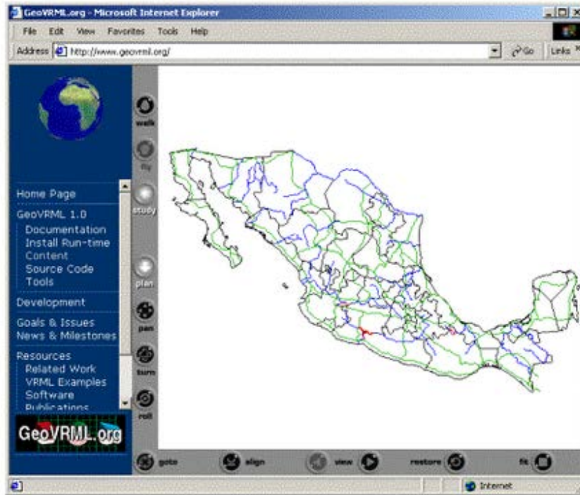
Figure 6. A GeoVRML translation of a Shape file produced by the ShapeViz utility from Bashir Research. This shows a number of layers for Mexico, including state boundaries, rivers, roads, lakes, and cities. This is being displayed in ParallelGraphics' Cortona 3.1 browser. Model provided courtesy of Bashir Research.
