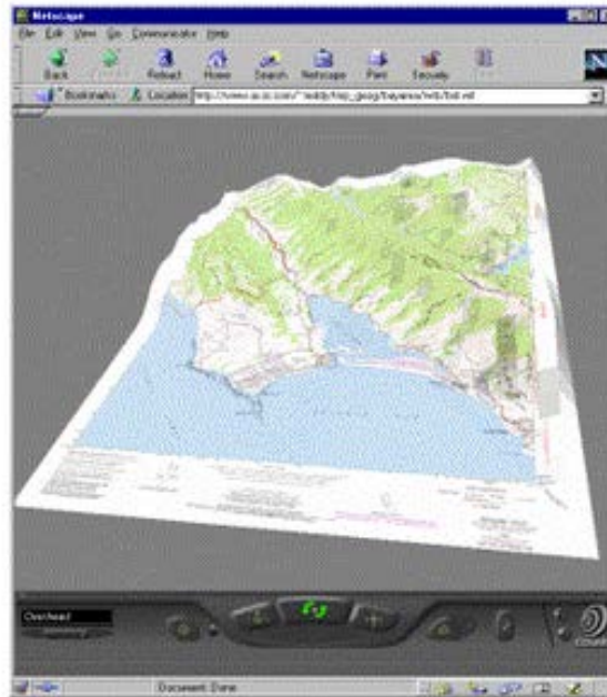
Figure 7. A USGS DEM that has been converted to a GeoElevationGrid using the dem2geog utility, and then draped with a DRG image for the same area.
