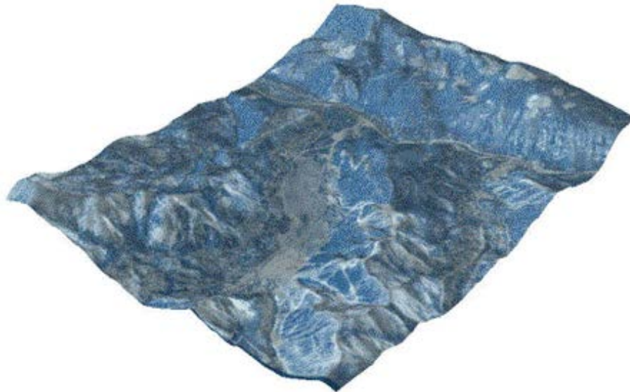
Figure 5. A GeoVRML model of Squaw Valley, CA, output by ESRI's ArcInfo 8.1 product (with 3D Analyst Extension). Model provided courtesy of ESRI.
