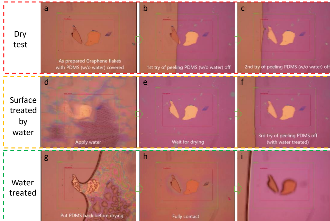
Figure 4.7 Screenshots of a supporting information video. a-c , a piece of dry PDMS cannot pick up graphene flakes from the substrate. d-f , after water changed the surface conditions of PDMS and substrate, the flakes still cannot be picked up. g-i , when a thin water film is sandwiched between PDMS and sample substrate, the graphene flakes are picked up by the PDMS and start to move out of the microscope focus. Note that the meniscus line is still under focus in i .
