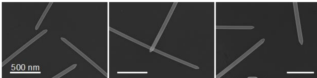
Figure 2.5 SEM images of purified ultra-sharp-tip AgNWs with an average diameter of 70 nm showing narrow diameter distribution and consistent tip morphology.
