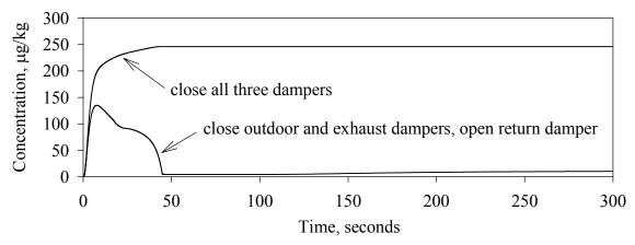
Figure 6: Concentration at the inlet of the supply duct for both actions.
