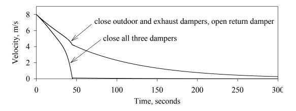
Figure 4: Velocity in supply duct for both actions.
