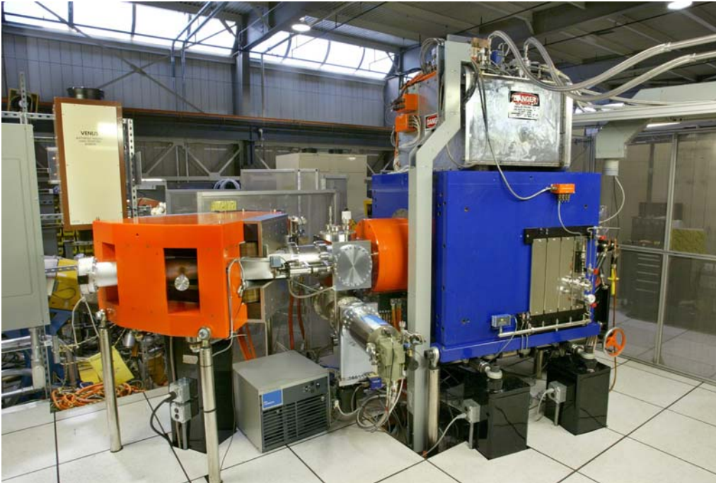
Fig. 1. VENUS ECR ion source installed on the vault roof of the 88-Inch Cyclotron.
