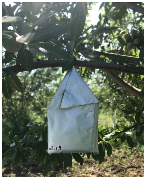
Top left: Acclima TDR probes (at 5 cm depth) connected to DataSnap solar datalogger. Top right: Phytech soil moisture probe. Bottom left: Phytech dendrometer attached to trunk. Bottom right: stem water potential bag around a leaf.
