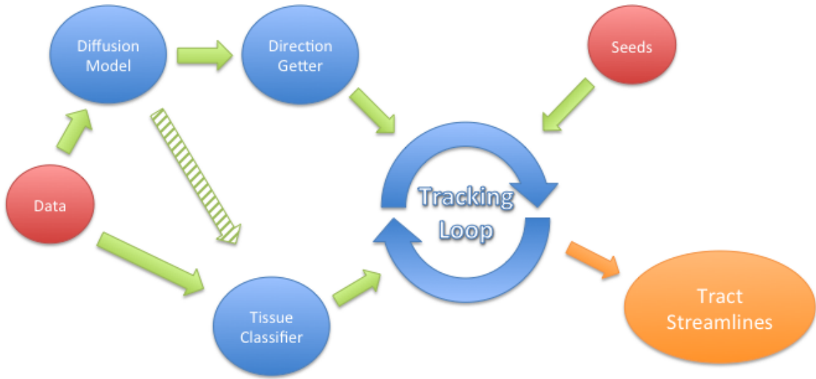
Figure 4.3: The organization of the local tracking components. Green arrows denote inputs into tracking components.
