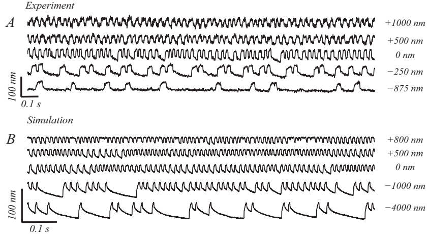
Figure 3.9: Effects of steady-state offsets imposed on an oscillating hair bundle. (A) Experimental records, where constant deflections were imposed on the bundle via a glass probe of stiffness 100 \mu\text{N/m} . (B) The corresponding numerical simulation. For offsets in the positive direction, the oscillations are faster and smaller and the quiescent intervals disappear. In the negative direction, however, the quiescent intervals occur more frequently and eventually become the dominant component of the oscillation profile. Parameters used in the simulation are those of Cell 1 in Table 3.1.
