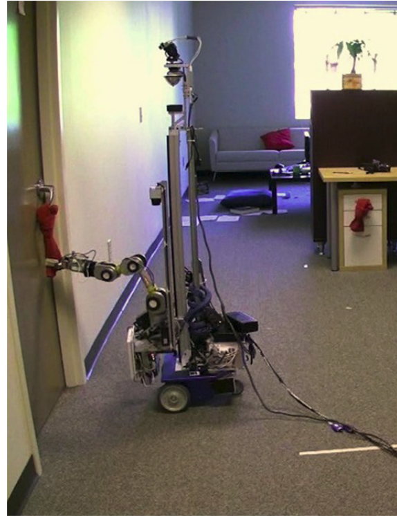
Fig. 6 On the left, the composition of the assistive heal care robot. On the right, the assistive robot helps the user to open a door with the handle tighten with a colored towel.
