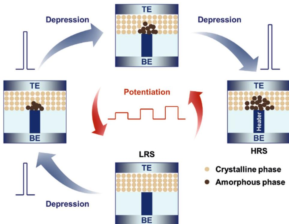
**Figure 5.** Bidirectional electric-induced conductance controllability for synaptic simulation. Normally, synaptic potentiation is obtained by lower and wider pulse and synaptic depression is achieved using higher and narrower pulse.
