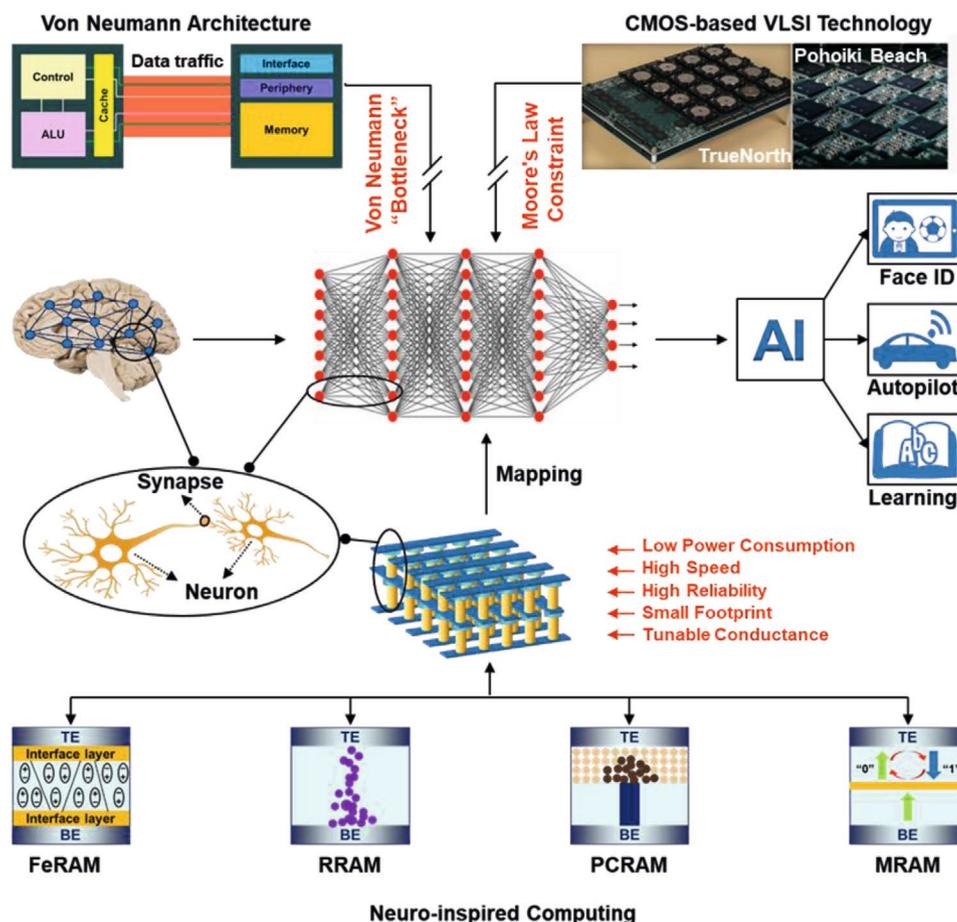
**Figure 1.** Introduction of neuro-inspired computing. Neuro-inspired computing based on memristors with integration of storage and computation avoids data traffic, becoming a promising alternative to emulate biological synapse, neuron, and BioNN.
