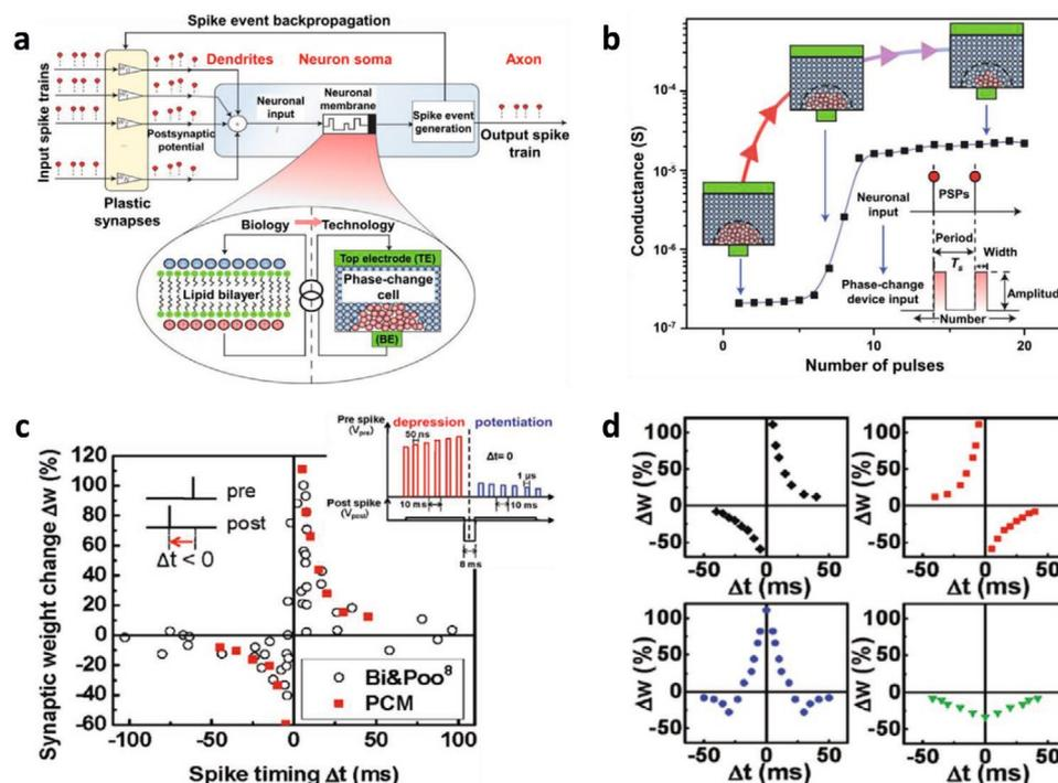
**Figure 6.** PCRAM neuronal system and synaptic simulation. a) Schematics of PCRAM electronic neuron and b) corresponding update of conductance to mimic LIF rule in biological neuron. Reproduced with permission.<sup>[66]</sup> Copyright 2016, Spring Nature. c,d) Four forms of STDP are simulated by regulating the intervals and amplitudes of programmable staircase pulse scheme in presynaptic spike. Reproduced with permission.<sup>[6]</sup> Copyright 2011, American Chemical Society.
