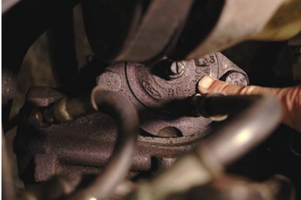
Figure 5: Steering gearbox showing hoses added to rack piston cylinder.
