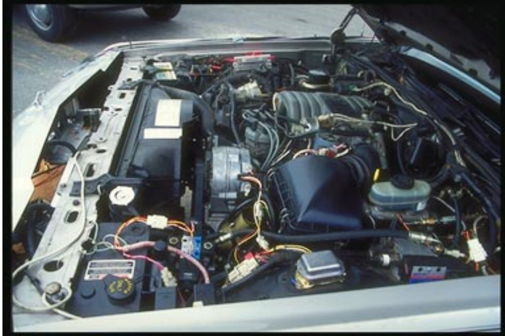
Figure 1: View of the left side of the engine compartment showing minimal disruption of the stock configuration. The only changes are removal of the cold air intake duct and removal of the original vacuum operated cruise control.
