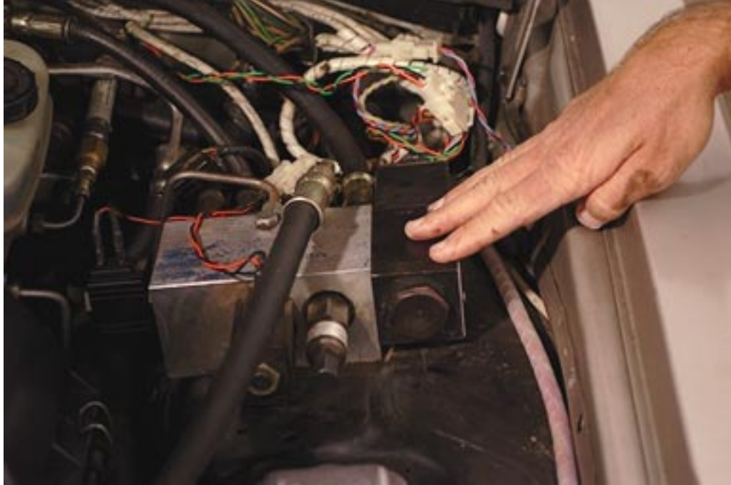
Figure 3: Figure 3. The brake manifold block, looking toward the rear of the car.
