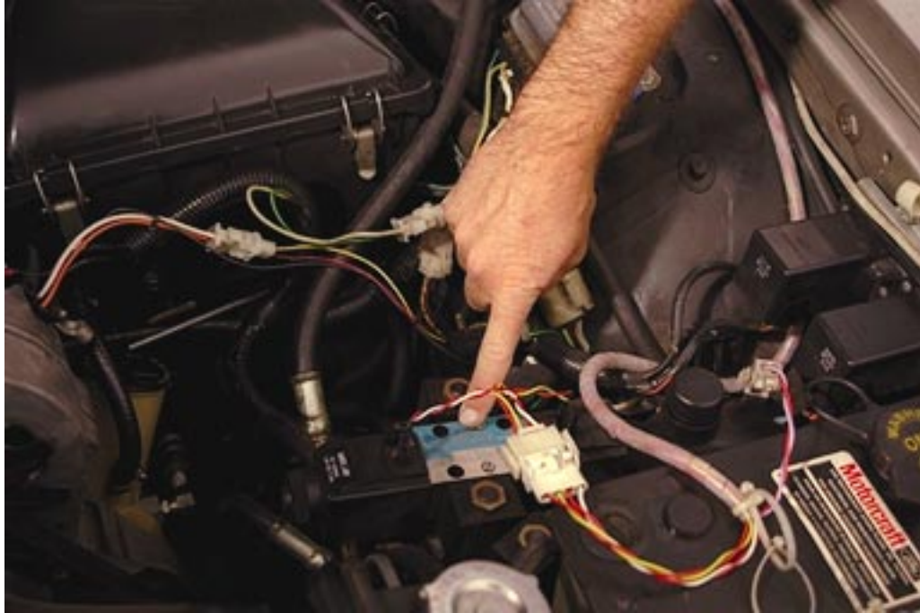
Figure 4: The steering actuator control valve, viewed from the front of the car. The manifold block extends about 4 inches below the control valve.
