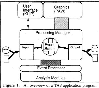
Figure 1. An overview of a TAS application program. Experiment specific routines are in the analysis modules section.
