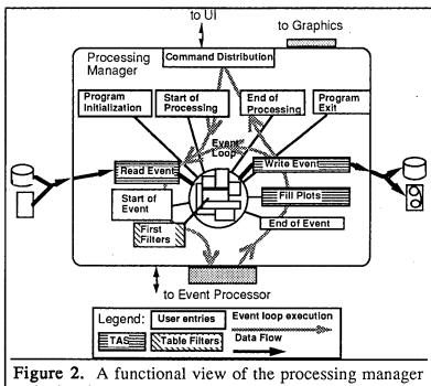
**Figure 2.** A functional view of the processing manager unit showing user entries and the I/O parts of the event loop.
