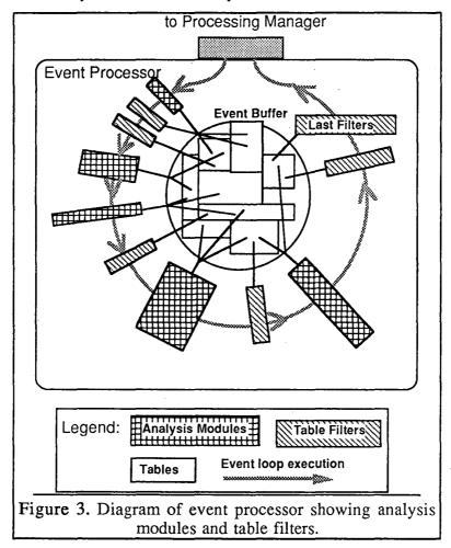
When the EP gets an event it compares the list of input tables to the list of tables requested for output (for either plot filling or saving into an output file) and uses the declared analysis module - table dependencies to determine which analysis modules to call in order to process the current event. This automatic mode of calling analysis
