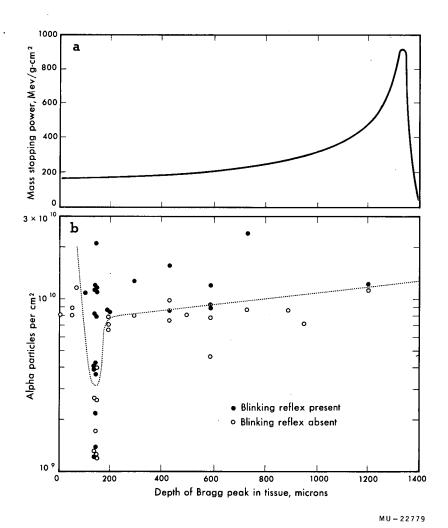
Fig. 5. (a) Bragg ionization curve in tissue-equivalent material of 10.4±0.2 Mev/amu He<sup>4</sup> (calculated from unpublished data, Brustad and Lyman).
