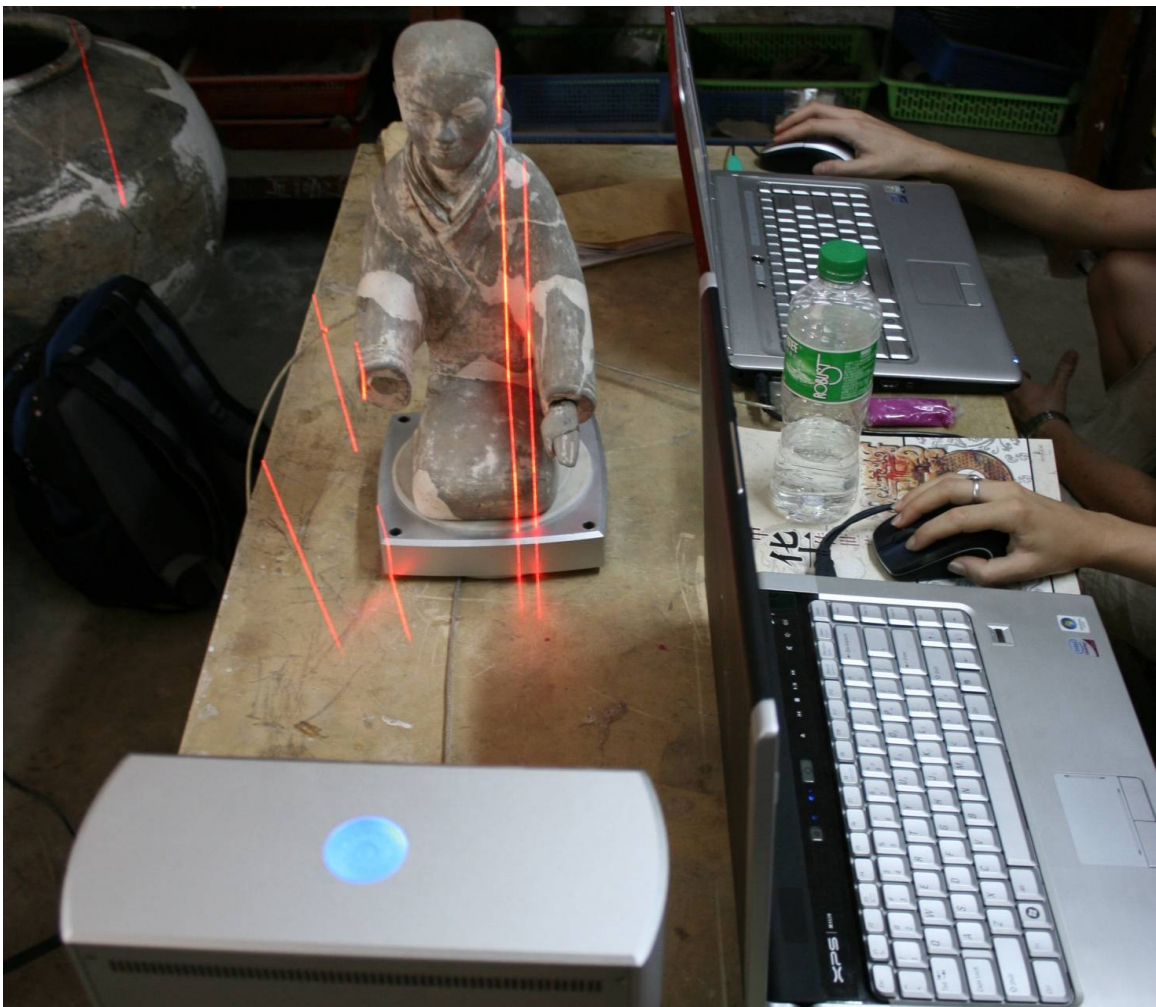
Figure 8. Laser scanning campaign of Western Han Dynasty artifacts. The laser scanning phase took place in a facility at the Xian Institute of Cultural Relics (© UC Merced).
