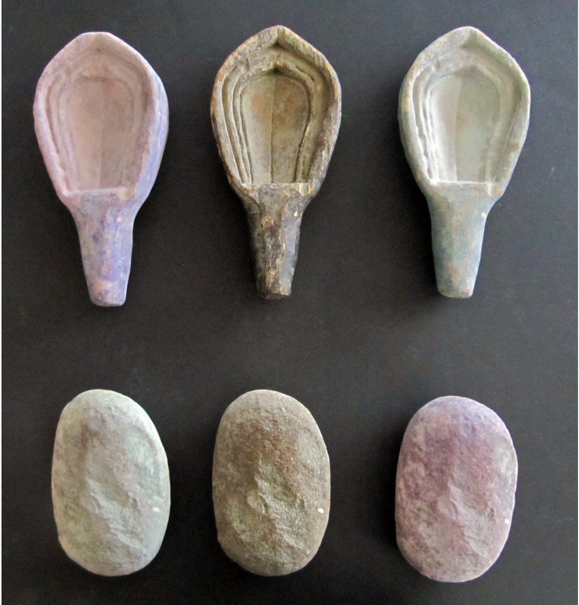
Figure 23. 3D prints of the Buddhist object and grinding stone. The original artifacts (in the center of the picture) in comparison to 3D printed copies made using a Zcorp.
