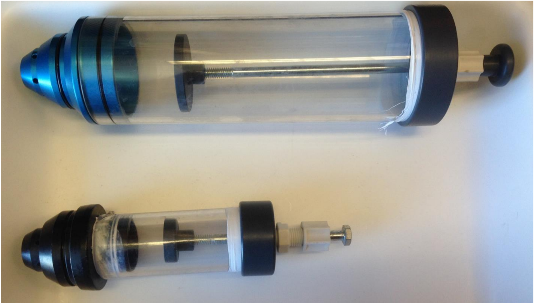
Figure 2.2a. Rat restraint tube with nose only port attached (top) compared to mouse restraint tube with nose only port attached (bottom).
