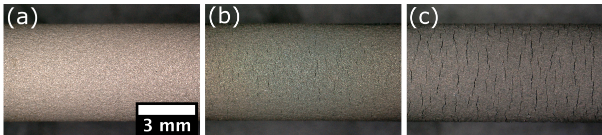
Figure 2.8: Optical micrographs from (a) TiNb-4 before testing (b) TiNb-4 interrupted at 25% of the fatigue life after 21.8 h of cycling ( N=39,297 ), and (c) TaNb-2 interrupted after 210.4 h of cycling ( N=378,734 )
