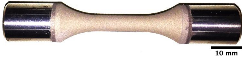
Figure 2.1: A CoNiCrAlY coated single crystal Co-base superalloy before low cycle fatigue testing.
