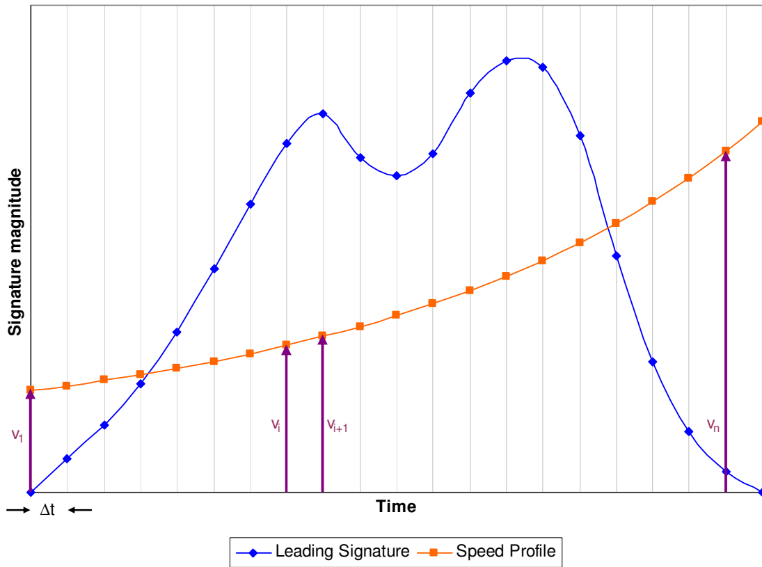
Figure 4.2. Obtaining the speed profile from sampled speeds spanning a vehicle signature
