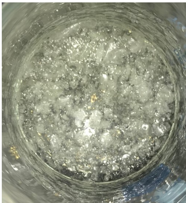
Figure 4.6: Chitosan and alginate crosslinked hydrogel using dicyclohexyl carbodiimide created irregularly shaped and waxy product.
