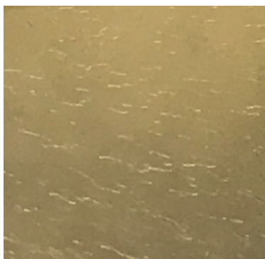
Figure 4.8: Hydrogel “skin” formed on surface of alginate stock when using humidifier to aerosolize \text{CaCl}_2 solution into alginate. Necessary to aerosolize alginate solution into \text{CaCl}_2 stock due to density difference allowing alginate particles to sink.
