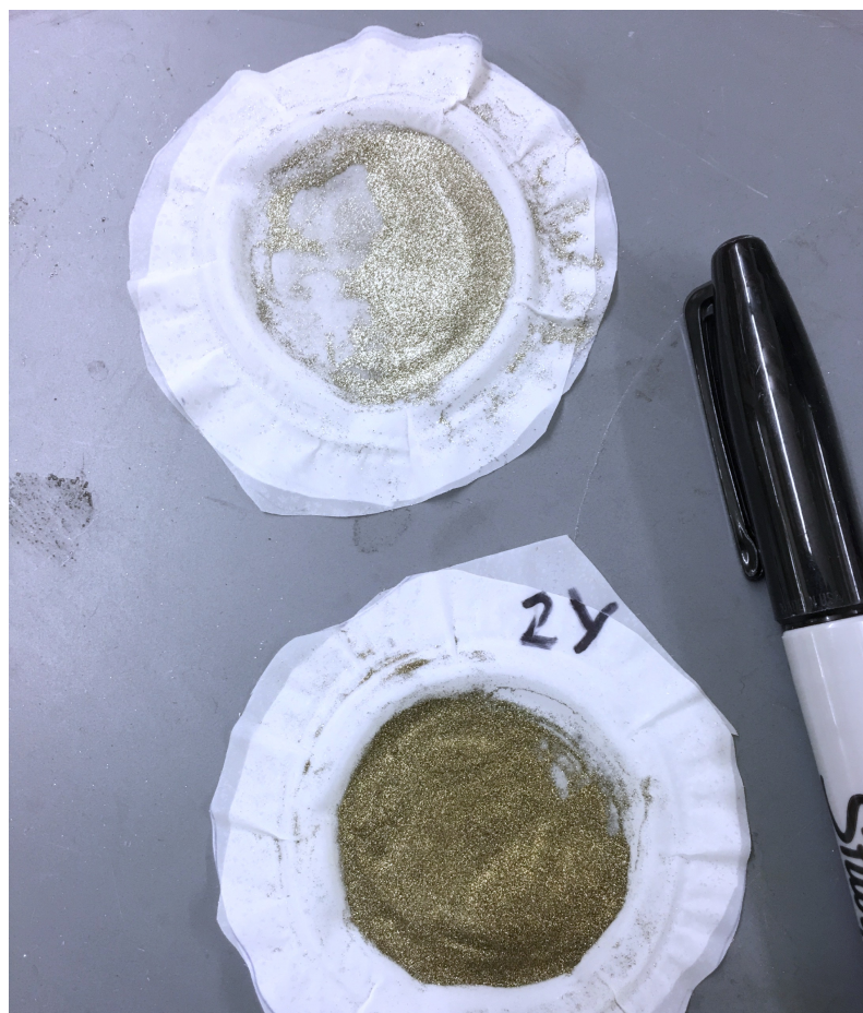
Figure 16. Pyrite on the top (oxidized at pH 2) looks unreacted. Pyrite on the bottom (oxidized at pH 8.1) is discolored, suggesting an iron ( \text{Fe}^{3+} ) hydroxide formed directly on the surface.
