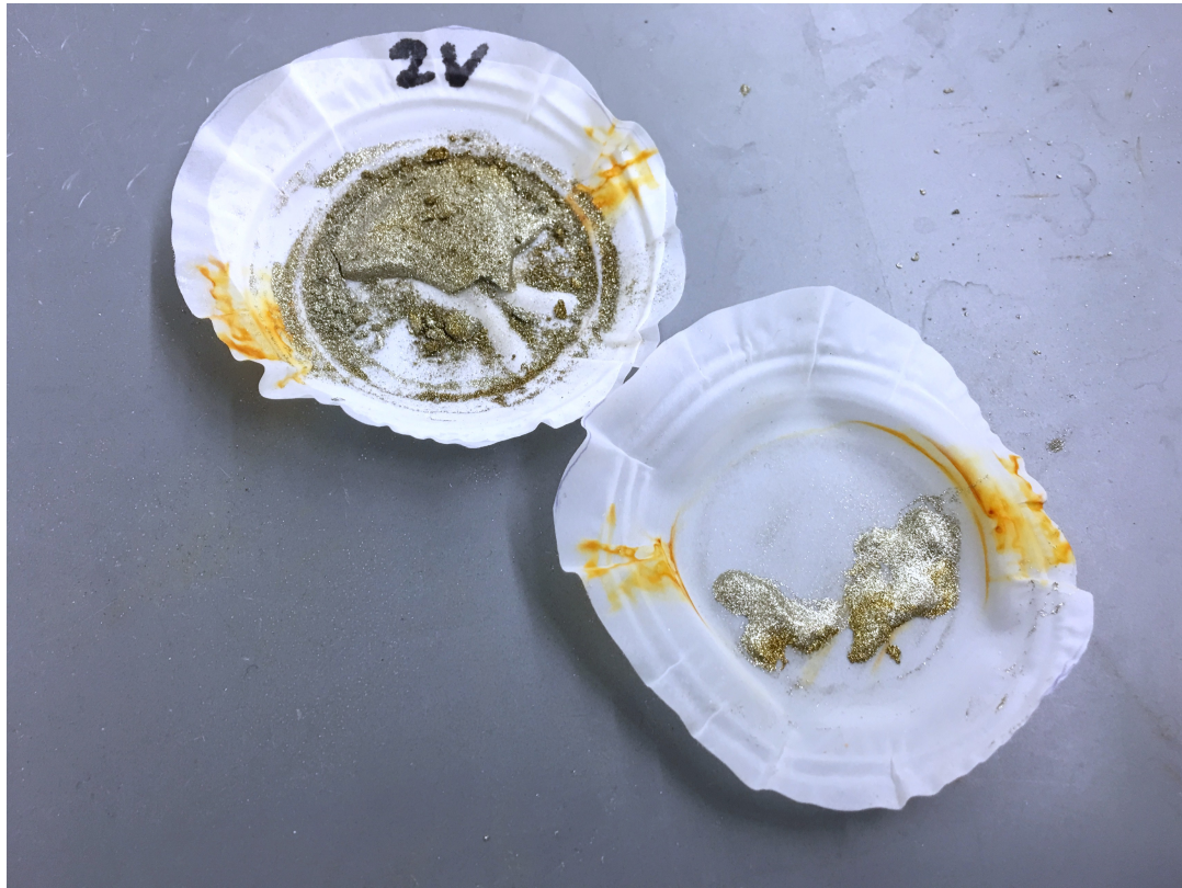
Figure 17. Sample-containing mesh after an experiment run at pH 5.5; an iron oxide precipitate has stained the mesh. This phenomenon was never observed under acidic conditions.
