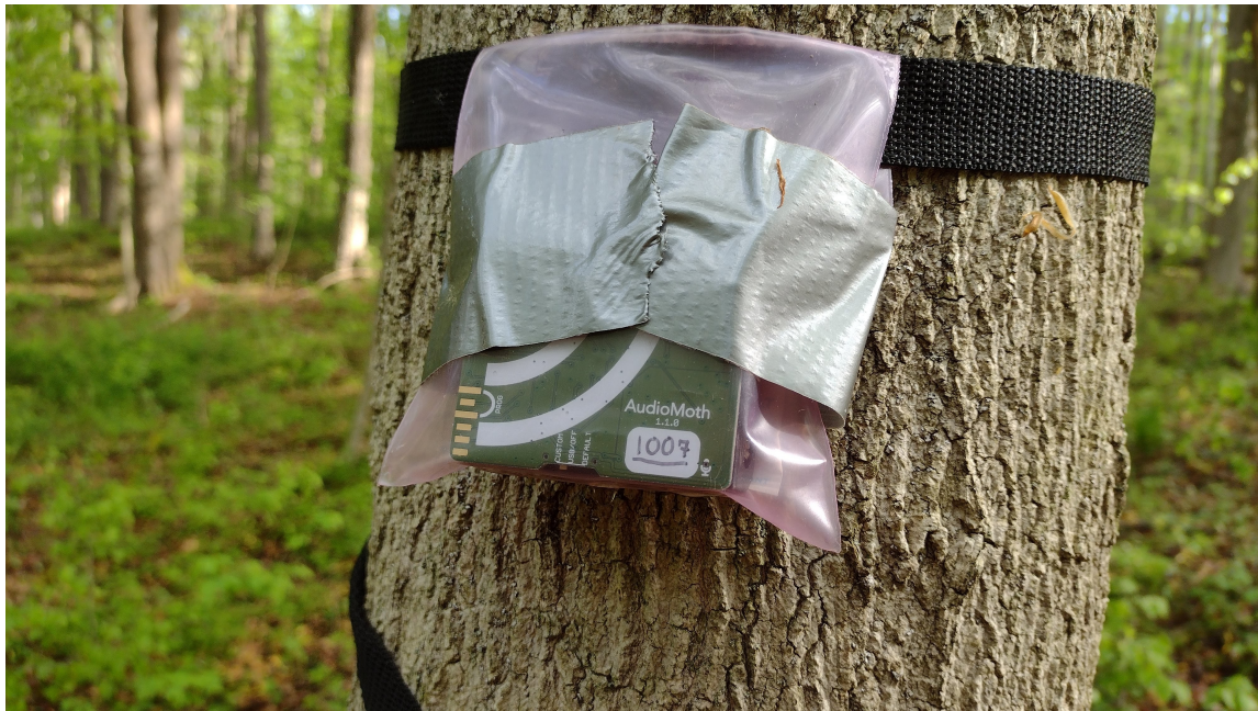
Figure 1: Autonomous Recording Unit at Pennsylvania Study Site. The ARU is placed in a plastic bag sealed with duct tape to avoid water damage and animal tampering and attached to a tree.
