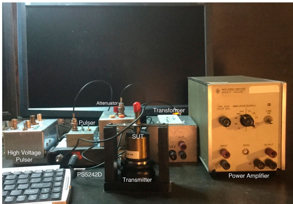
Figure 5. A photograph of the face-to-face test set-up.
