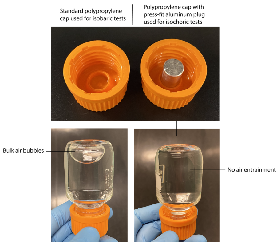
Figure 3.5: Cap modification to allow effective air removal in sealing of isochoric chambers. Left top: Standard polypropylene cap, as used for assembly of isobaric chambers. Left bottom: inverted chamber after assembly with standard cap. Bulk pockets of air can be observed. Right top: Polypropylene cap with press-fit aluminum plug, as used for assembly of isochoric chambers. As the cap is threaded onto the chamber, the plug displaces a small volume of water, which forces out any air remaining in the mouth of the chamber or trapped in the cap itself. This displaced liquid and air is able to escape past the threads as the cap is being tightened, until the final point of closure, at which the roof of the lid meets the lip of the chamber and forms a rigid seal. Right bottom: inverted
