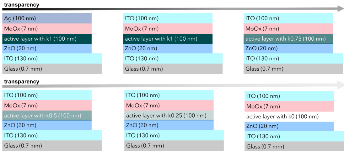
Figure S5.1. Device architectures of the solar cells studied by simulation in this work, related to Figure 5.1.
