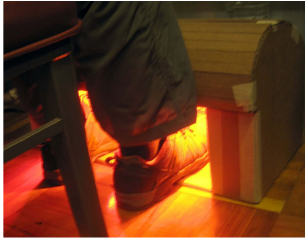
Figure 3.5: Early functional cardboard prototype of the final footwarmer shape being tested to refine dimensions and arrangement.
