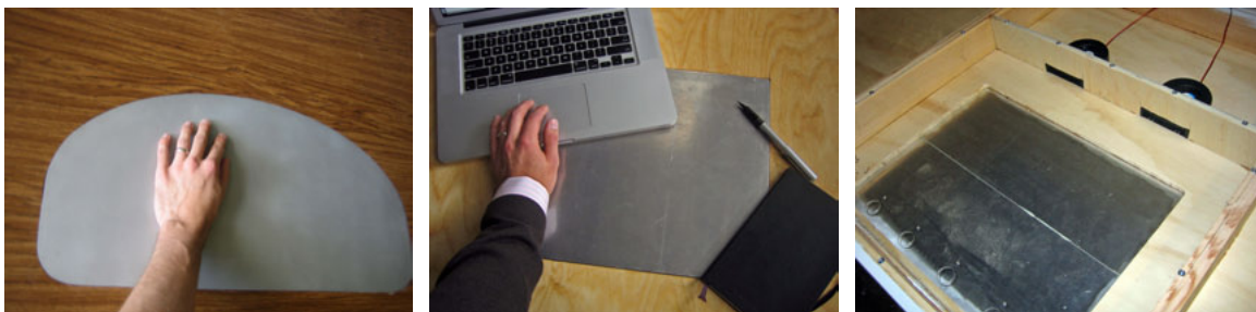
(a) Prototype desk with exposed conductive surface for cooling, and resistance heating. (b) Prototype desk with reversible conductive surface for passive cooling. (c) Underside of the desk showing the conductive surface and blower fans.
