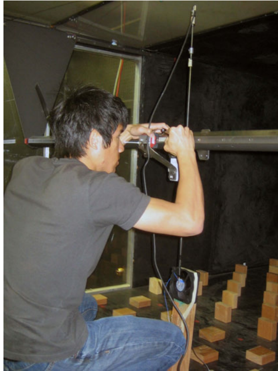
Figure 2.6: Research assistant Spencer setting up the anemometer gantry to measure the air-speed of various nozzles and inlets mounted on a standard fan to inform fan cowling design.
