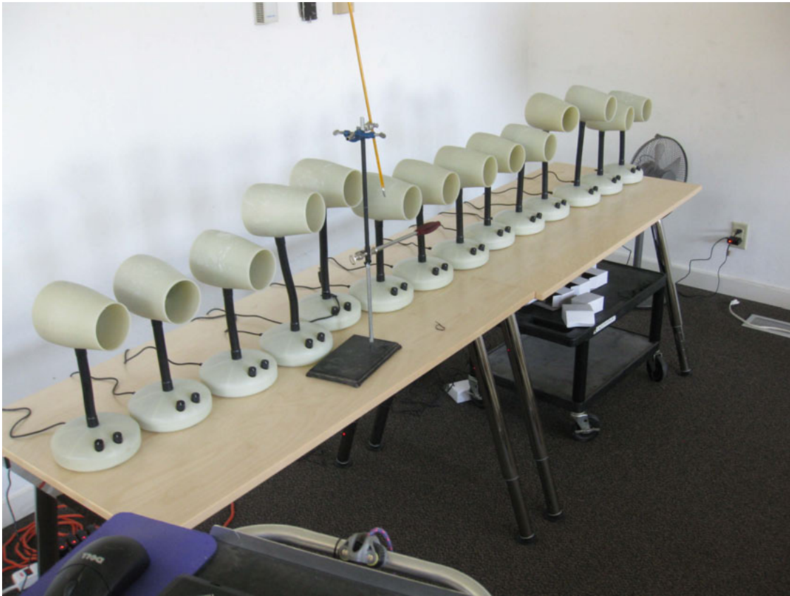
Figure 5.4: A random sample of fans arranged for calibration in the controlled environmental chamber. Note the mercury reference thermometer on its stand..
