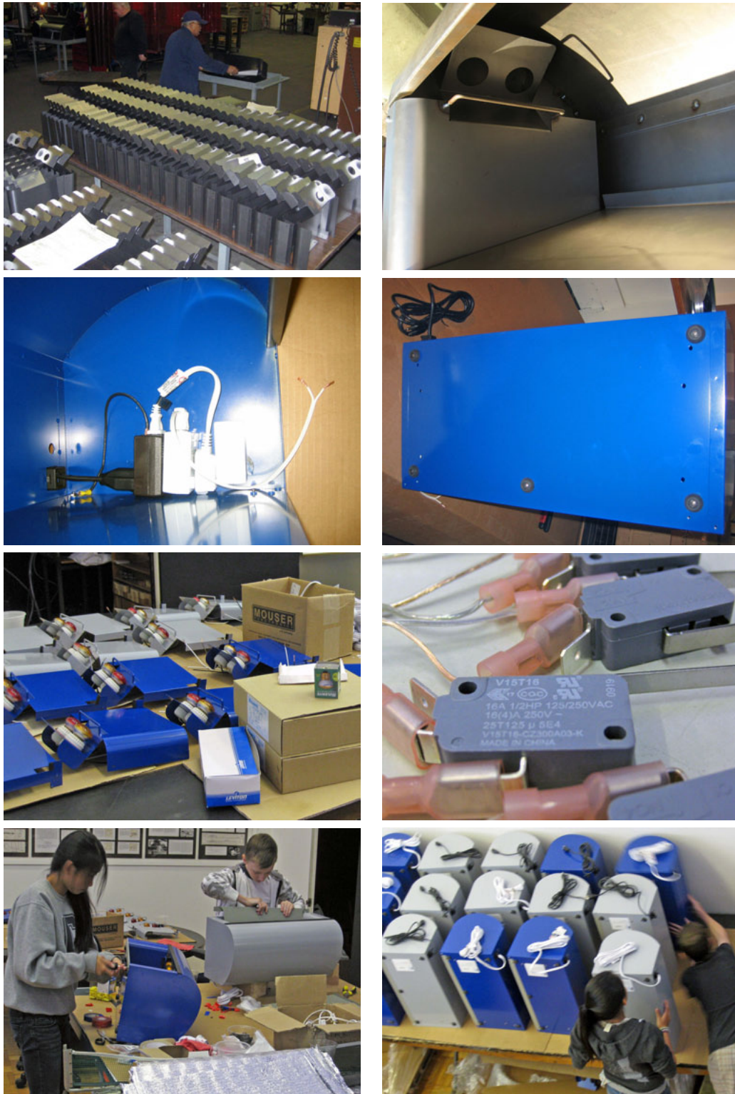
Figure 3.9: Images showing the fabrication, components and assembly of the footwarmer.
