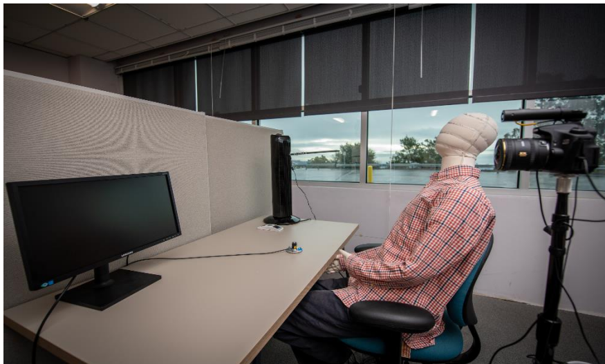
Figure 4. Photograph of window-adjacent workstation in test cell. This photograph shows the desktop illuminance sensor, as well as the HDR camera for sensing glare in the occupant field of view. The CorePlus automated shades are in use and, likely due to the cloudy sky condition, are retracted halfway to allow daylight into the space.
