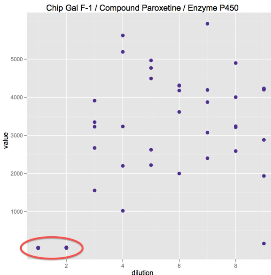
Figure 3.13: Example of experimental problem of edge bleeding.
