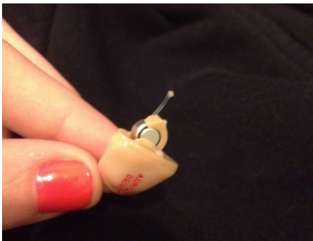
Image 1. An in-the-ear hearing aid similar to our patient's, in the off position with battery exposed.
