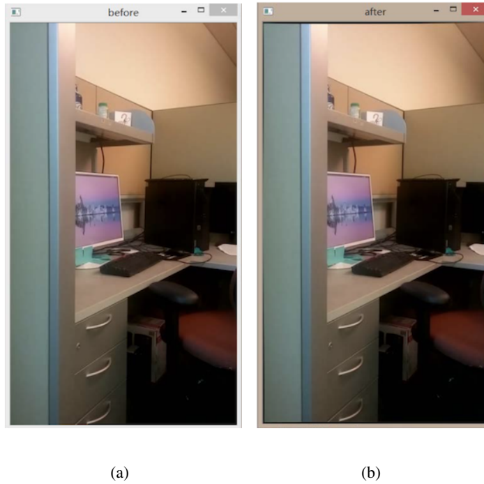
Figure 3.2: An image distortion correction example. The left image shows the original image, and the right image shows the result after distortion correction process.
