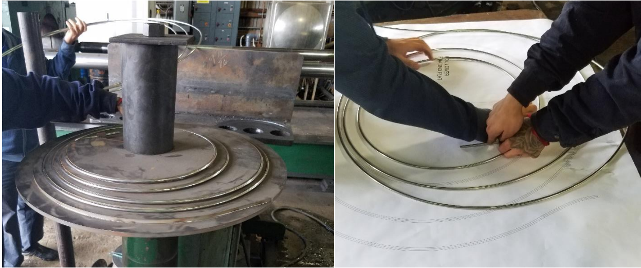
Figure 3-5. Bundle Fabrication: (Left) Tube Coil Die on Mandrel; (Right) Shaped by Hand to Match Drawing
