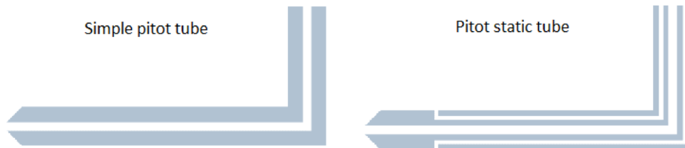
Figure 3-9. Schematic Diagram of Simple Pitot Tube (Left) & Pitot-Static Tube (Right)
