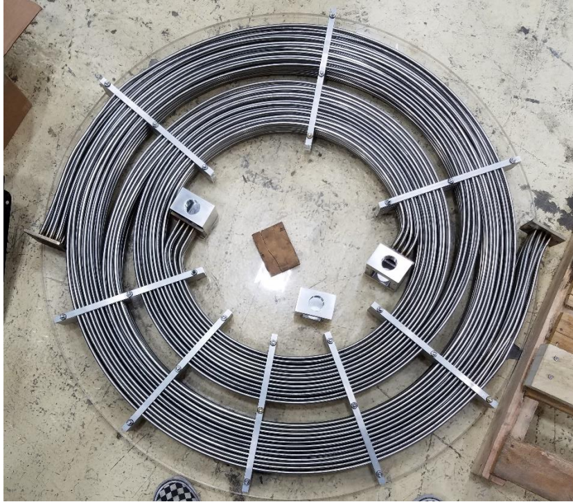
Figure 3-6. CASET Fabricated Tube Bundle
