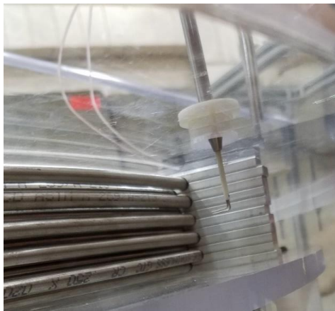
Figure 3-10. Hot-Wire Anemometer Probe Measurement
