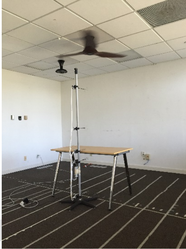
Figure 37: The ceiling fan in the chamber, and the velocity sensors
