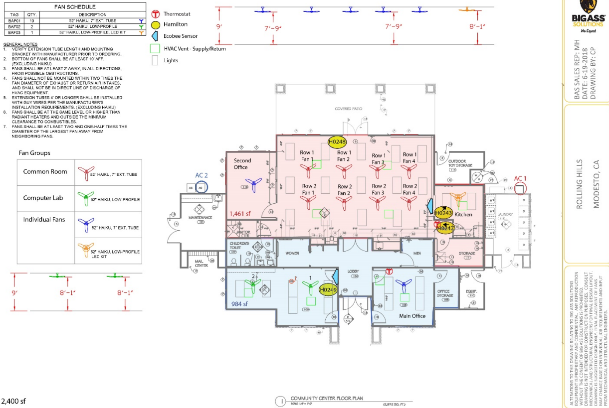
Layout of Rolling Hills Community Building demonstration site showing ceiling fan and thermostat locations, HVAC control zones, Hamilton temperature and humidity sensors, and lighting and HVAC vents.
