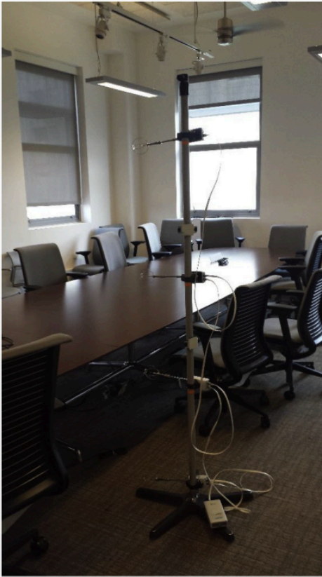
Fig. 1. The anemometer tree replacing a chair at a conference table.
