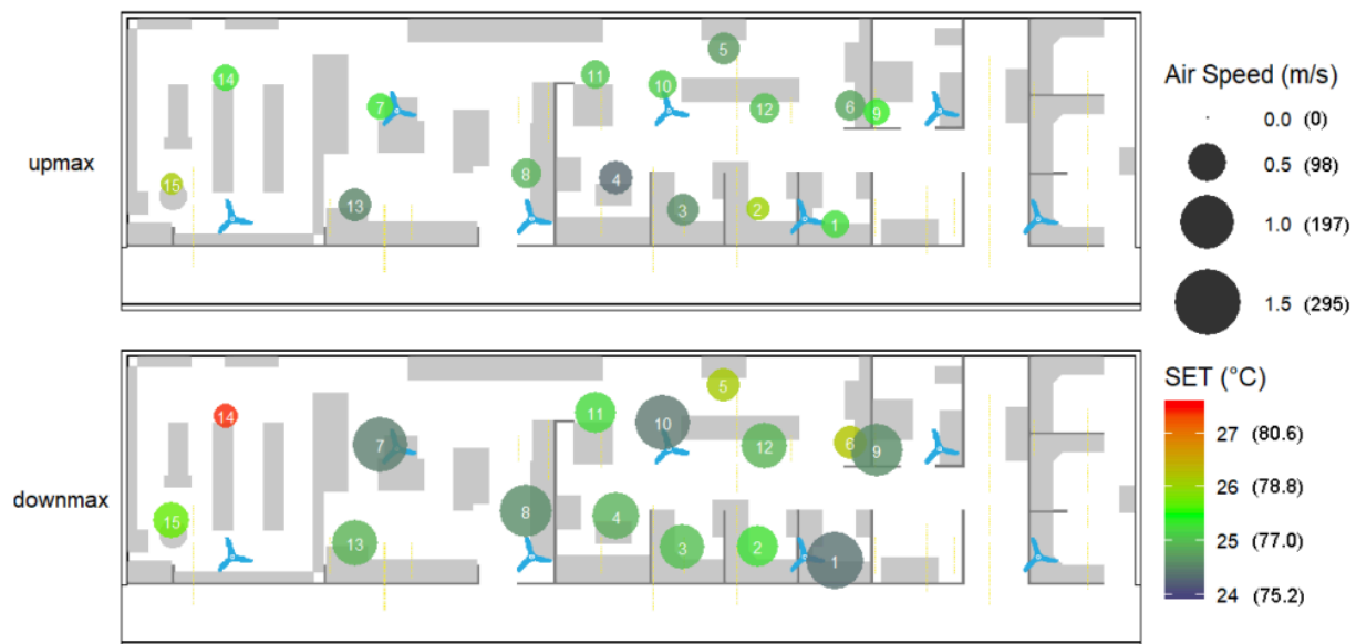
Figure 5 Mean SET and air speeds at each measurement site for the upmax (top) and downmax (bottom) test conditions. The SET calculation used an operative temperature corresponding to thermal neutrality based on the mean air speed of each test as a way to normalize the cooling effects of elevated air movement across the upwards and downwards blowing tests. The background is the floorplan showing the location of fans (blue symbols), office furniture (grey squares) and partitions (solid grey lines). Note the fan in the lower right was not able to be reversed
