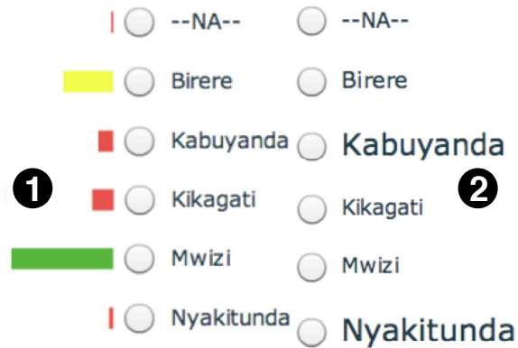
Figure 3.4. Alternative designs for radio button feedback: (1) radio buttons with bar-chart overlay. (2) radio buttons with scaled labels.
