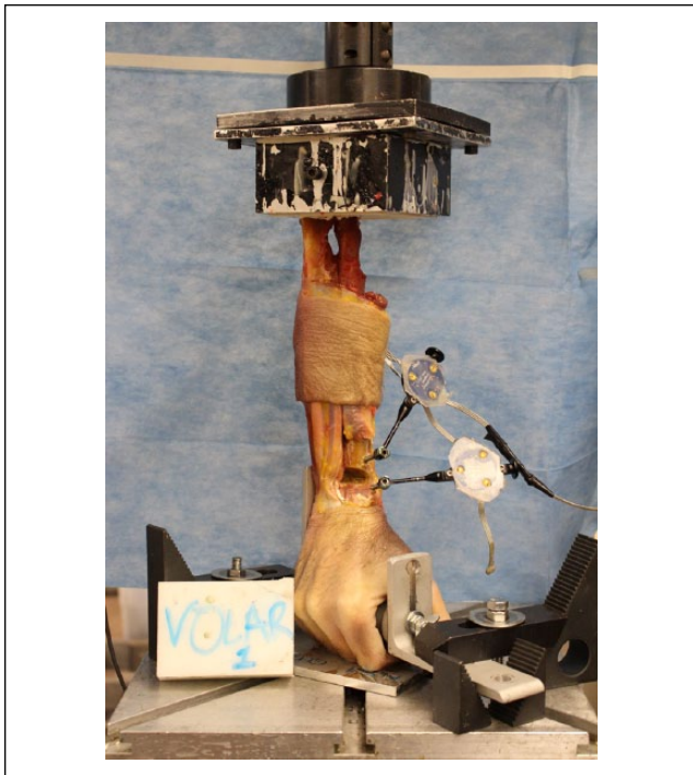
Figure 1. Biomechanical testing setup: The proximal was potted in resin and was attached to the MTS actuator and the hand was mounted to a crutch handle. Optical motion-tracking sensors were attached to the proximal and distal segments adjacent to the fracture site.
