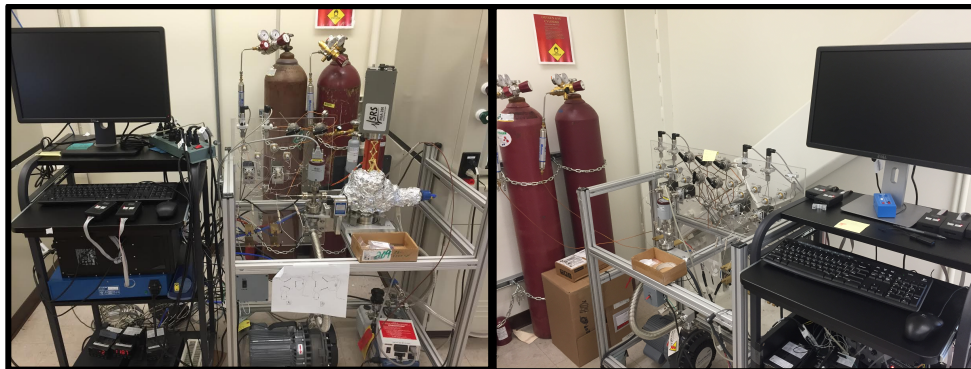
Figure 2.3. (Left) Two-channel pressure monitoring and differential electrochemical mass spectrometry (DEMS) battery cell testing system. (Right) Five-channel pressure monitoring battery cell testing system.
