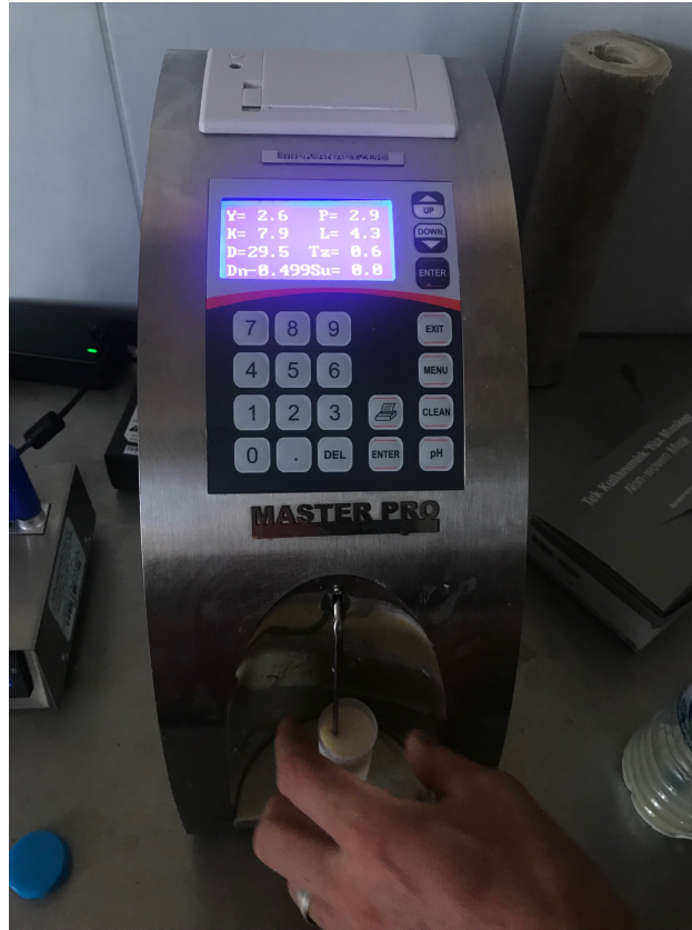
Photograph 8: A milk analyzer machine in a small dairy in Boğatepe village (2018).
