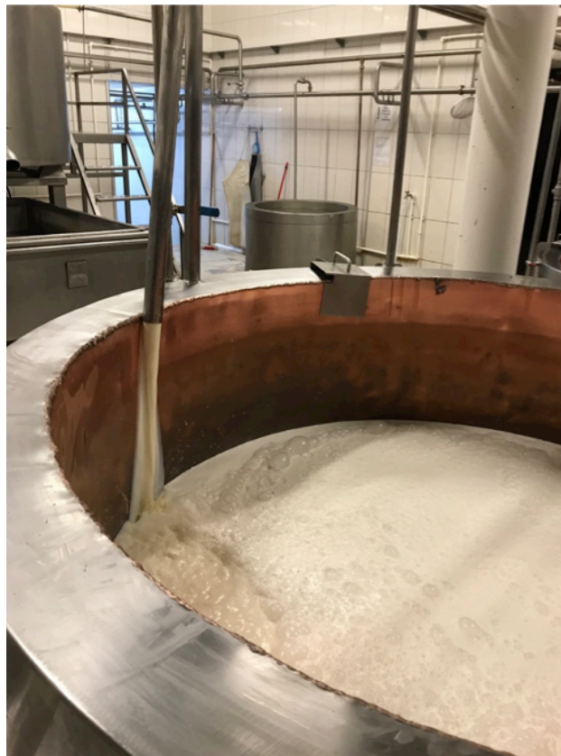
Photograph 14: The milk, passing through the tubes, fills the cauldron undercover in the new zavot (Boğatepe, 2018).
